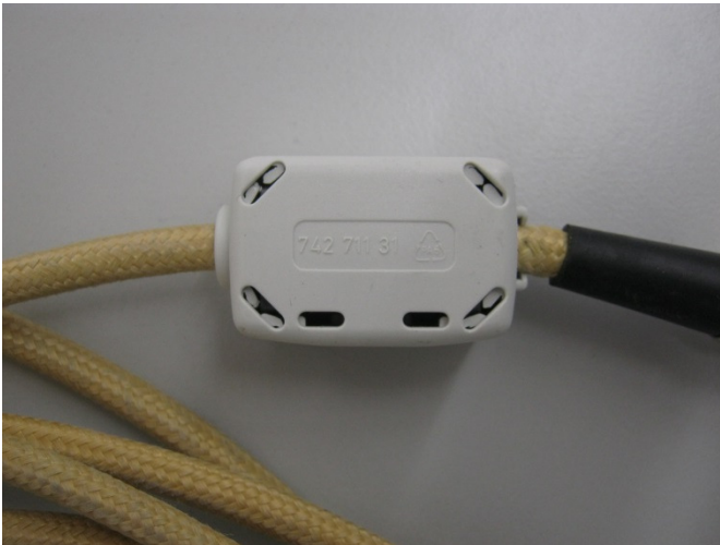
Photograph 2.3-7: Detailed view on ferrite Würth (742 711 31) on connection cable
