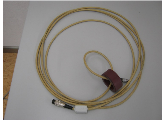
Photograph 2.3-6: Connection cable from Axon Control Unit to Axon Stator Unit with ferrites
