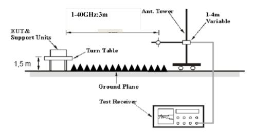
The radiated emission and out of band emission tests were performed in the 3 meters chamber test site, using the setup accordance with the ANSI C63.10-2013 The specification used was the FCC 15.209/15.205 and FCC 15.255 limits.
