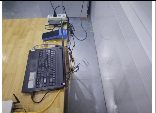
Conducted Emissions Test Setup – Side View
