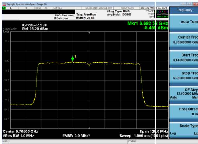
Plot 7-304. Power Spectral Density Plot Antenna WF8 LPI (80MHz 802.11ax (UNII Band 7) – Ch. 151, MCS4)
