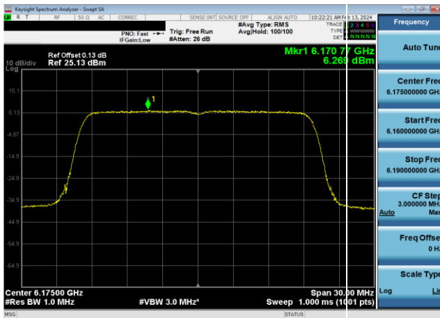
Plot 7-333. Power Spectral Density Plot Antenna WF8 Standard Power (20MHz 802.11ax (UNII Band 5) – Ch. 45, MCS2)
