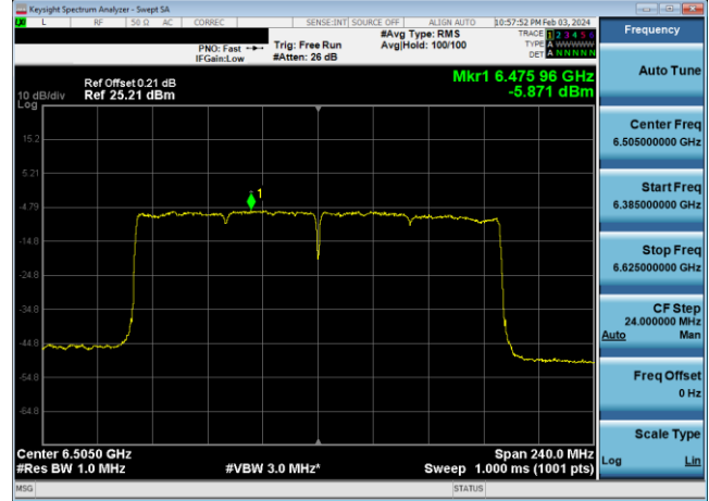
Plot 7-300. Power Spectral Density Plot Antenna WF8 LPI (160MHz 802.11ax (UNII Band 6) – Ch. 111, MCS4)
