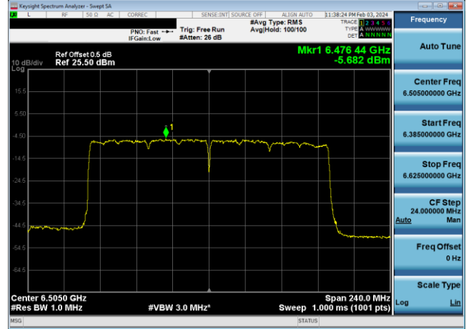
Plot 7-320. Power Spectral Density Plot Antenna WF8 LPI (160MHz 802.11ax (UNII Band 6) – Ch. 111, MCS11)
