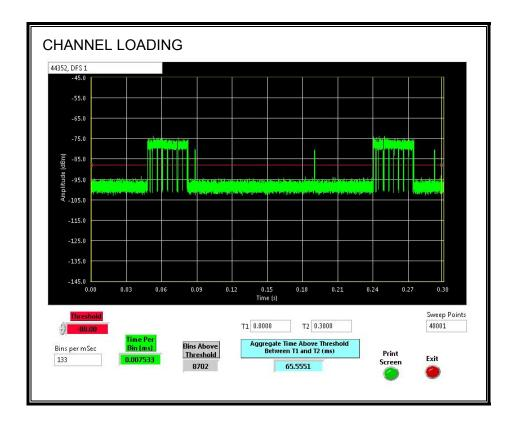
The level of traffic loading on the channel by the EUT is 21.85%
