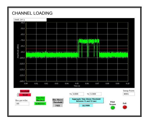
The level of traffic loading on the channel by the EUT is 18.8%
