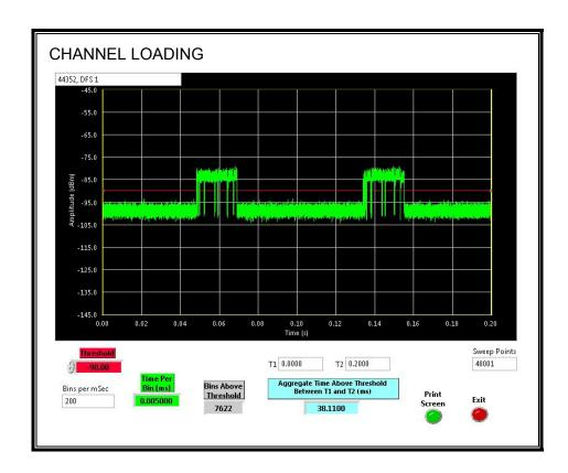
The level of traffic loading on the channel by the EUT is 19.055%
