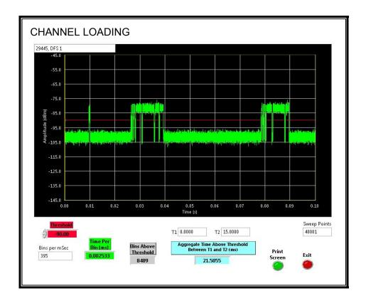
The level of traffic loading on the channel by the EUT is 21.5%
