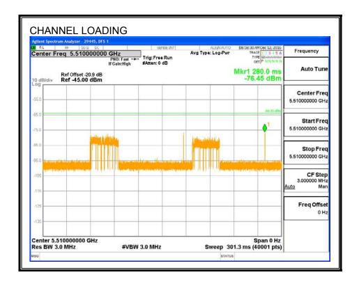
The level of traffic loading on the channel by the EUT is 20.92%
