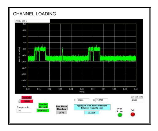
The level of traffic loading on the channel by the EUT is 19.19%
