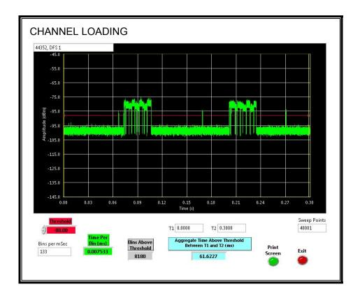
The level of traffic loading on the channel by the EUT is 20.54%
