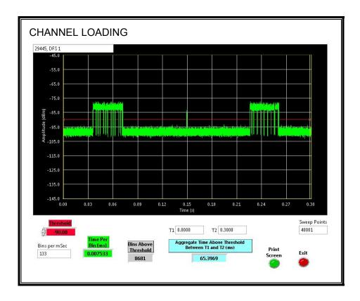
The level of traffic loading on the channel by the EUT is 21.78%
