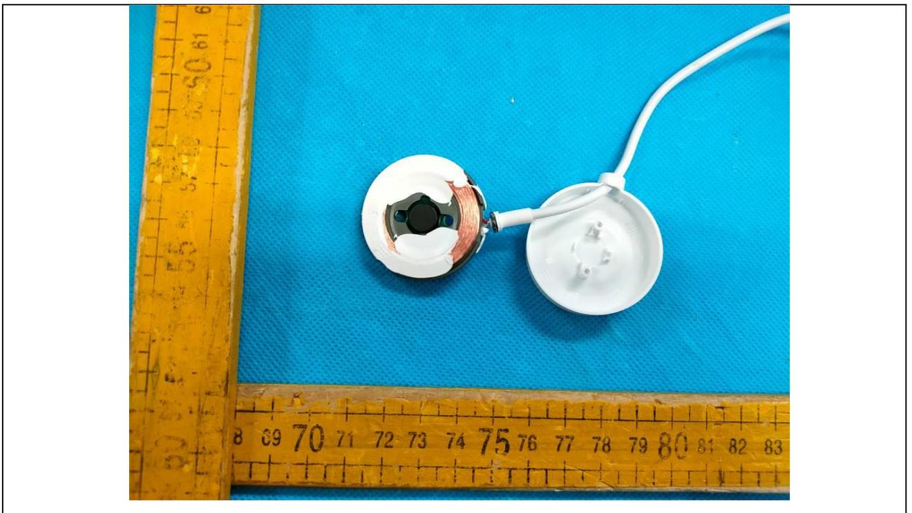
Details of: PCB and coil view 1
