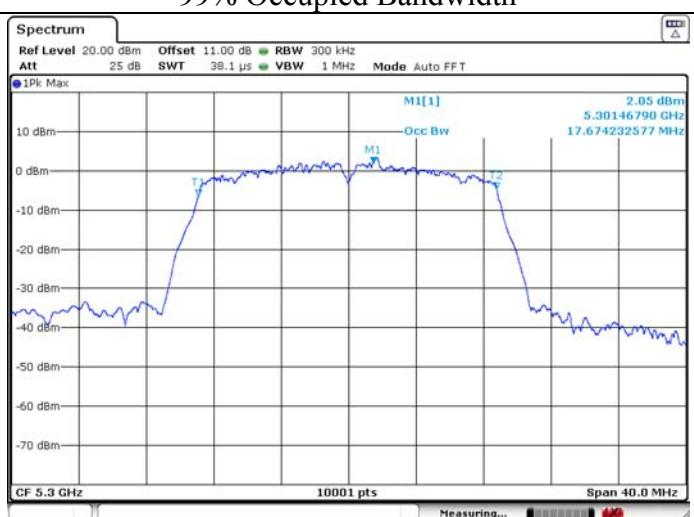
**U-NII-2A IEEE 802.11ac VHT20 5320MHz****26dB Bandwidth**
