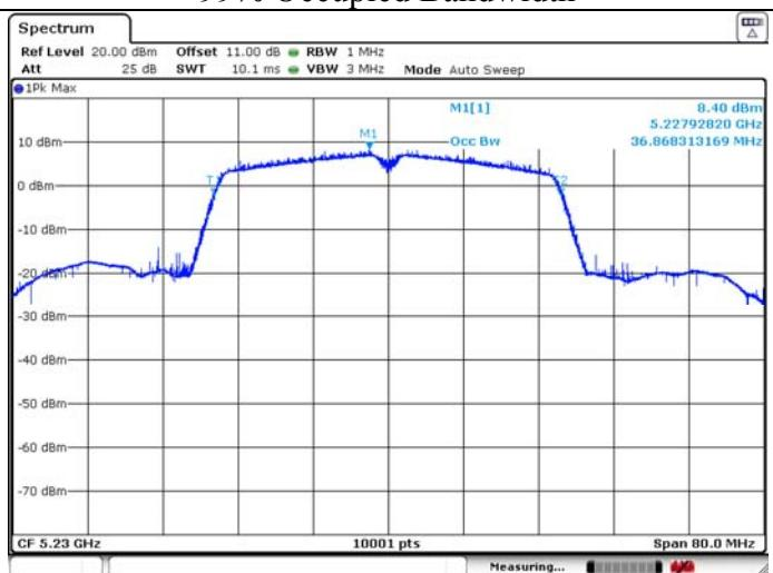
**U-NII-1 IEEE 802.11ac VHT40 5190MHz****26dB Bandwidth**
