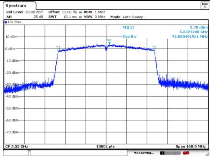
**U-NII-2C IEEE 802.11ac VHT80 5610MHz****26dB Bandwidth****99% Occupied Bandwidth**
