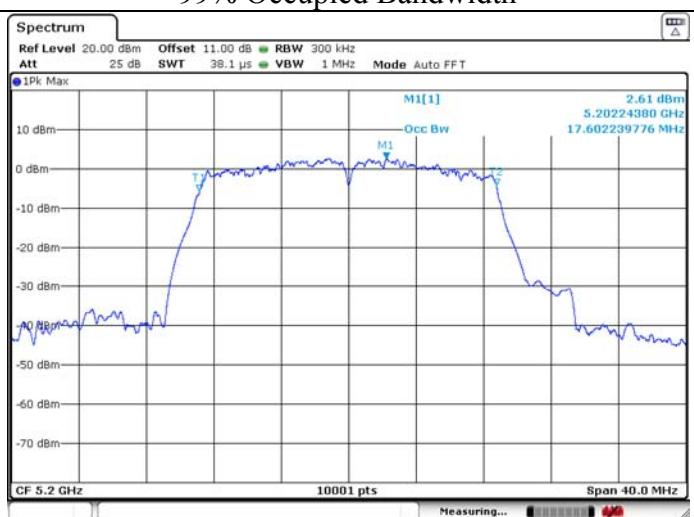
**U-NII-1 IEEE 802.11ac VHT20 5240MHz****26dB Bandwidth**
