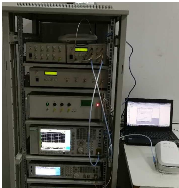
Photograph 2: Setup for Spurious emissions, 30MHz-1GHz
