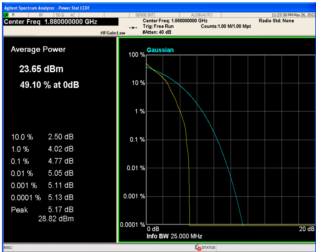
Band2 QAM16 BW=1.4MHz Channel=18900 RB Size=1 Position=#0
