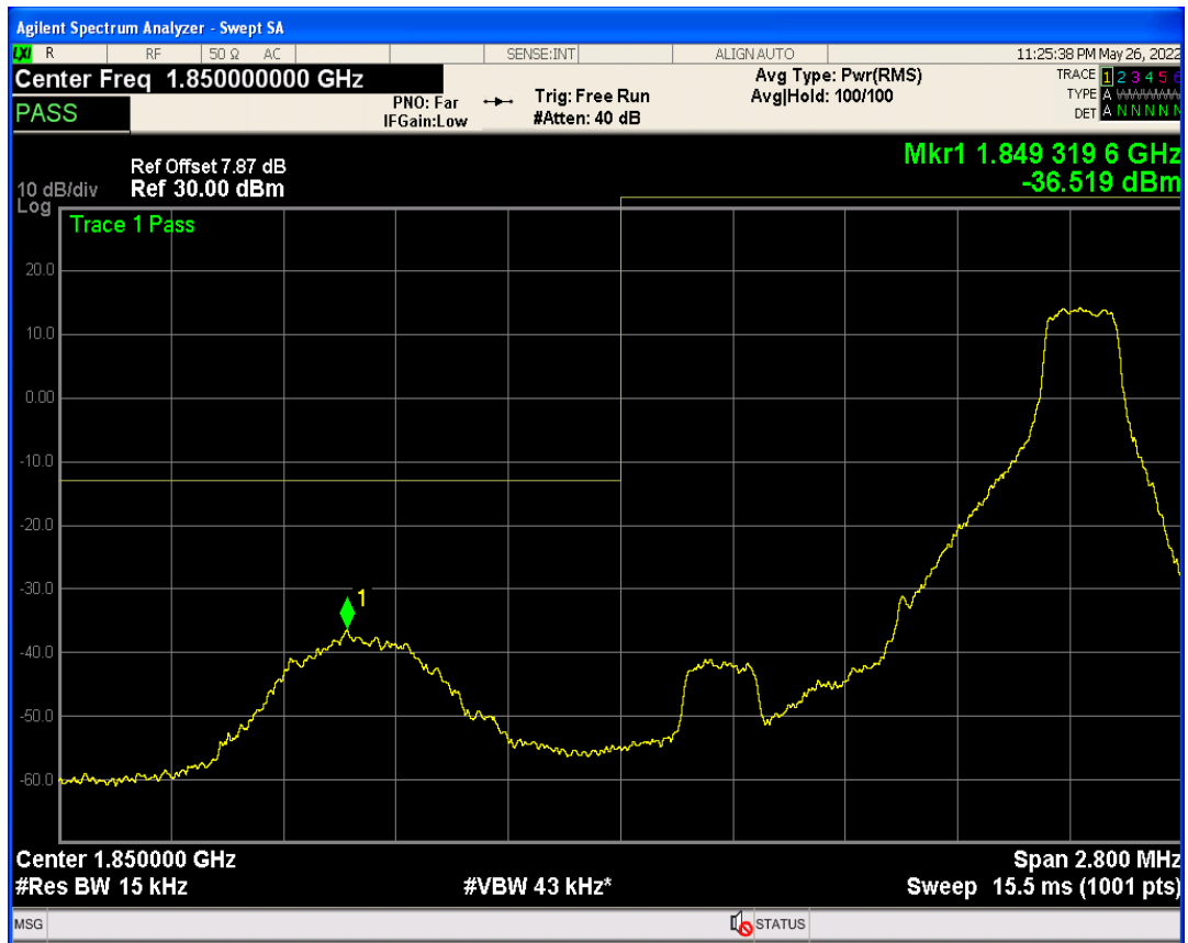
Band2 QPSK BW=1.4MHz Channel=18607 RB Size=1 Position=#0
