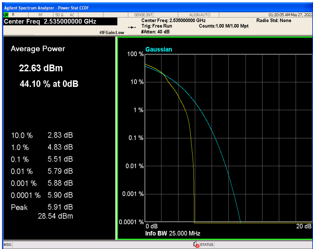
Band7 QPSK BW=20MHz Channel=21100 RB Size=1 Position=#0
