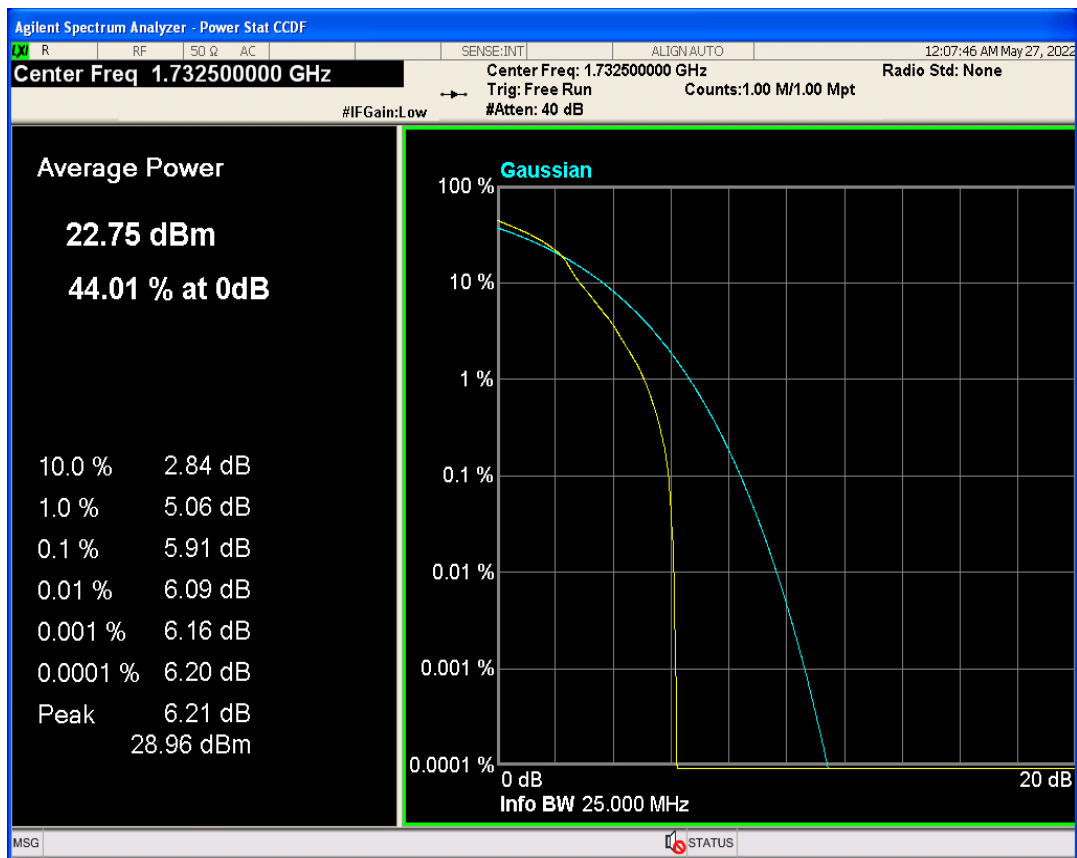
Band4 QPSK BW=5MHz Channel=20175 RB Size=1 Position=#0
