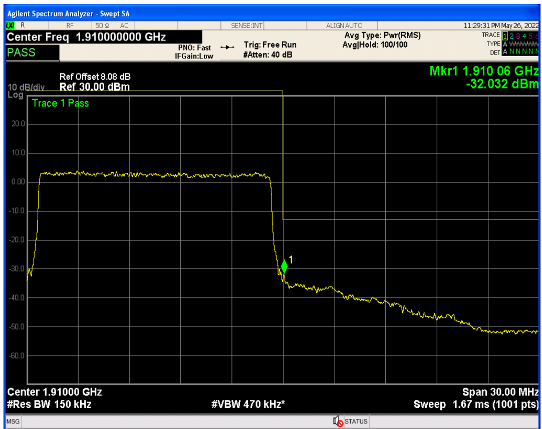
Band2 QPSK BW=20MHz Channel=18700 RB Size=1 Position=#Max
