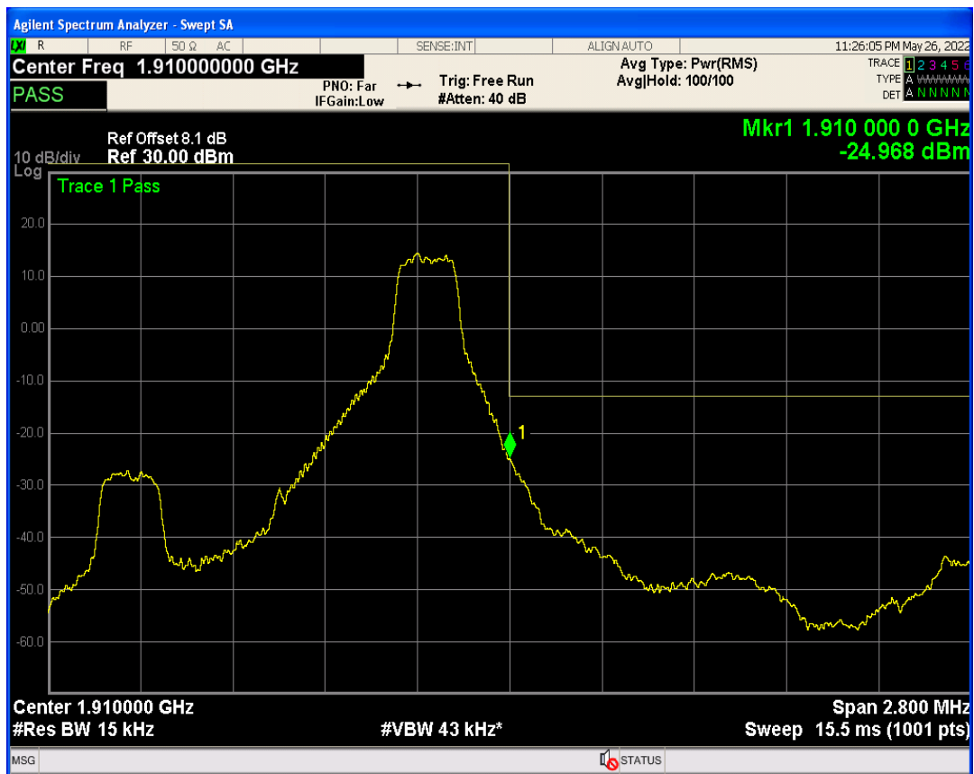
Band2 QPSK BW=1.4MHz Channel=19193 RB Size=6 Position=#0
