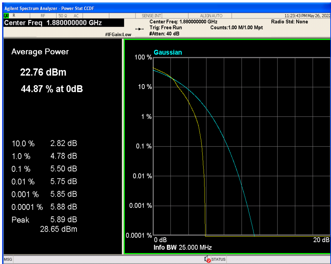
Band2 QPSK BW=5MHz Channel=18900 RB Size=1 Position=#0
