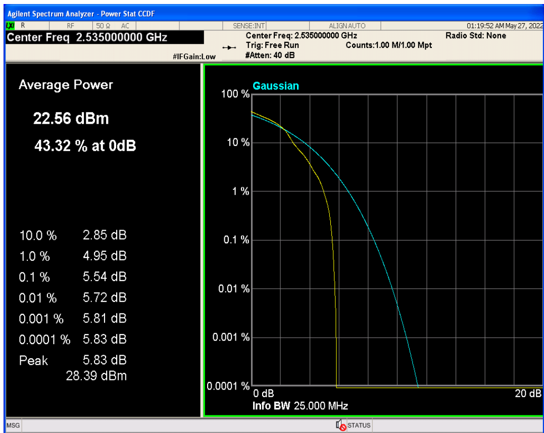
Band7 QPSK BW=15MHz Channel=21100 RB Size=1 Position=#0
