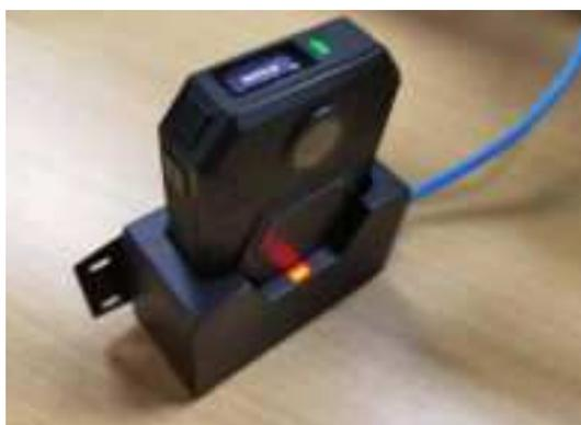
Step 3. When a BWC is not fully charged yet, the status light is blinking green. After the BWC is fully charged, the status light turns solid green.
