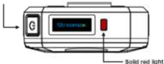
Step 2. When the BWC status light turns from solid red to solid green, and the logo on the LCD disappears and changes to the BWC status, the BWC is powered on and in standby mode.
