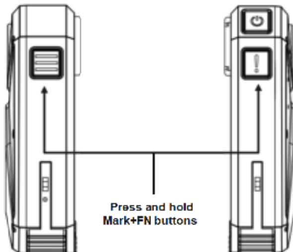
Step 2. When **ENTER STEALTH MODE** is displayed on the LCD, wait for 5 seconds until the notification disappears. The BWC enters stealth mode.
