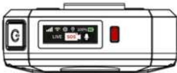
Step 4. A "LIVE" icon is displayed on the left side of the LCD, as shown in the following figure. This icon will be displayed until the platform monitoring or BWC recording is stopped.
