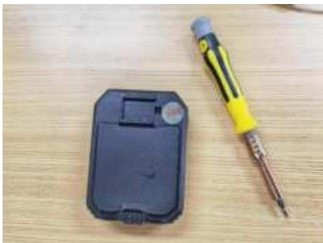
Step 2. Open the rear cover of the BWC and take out the battery.
