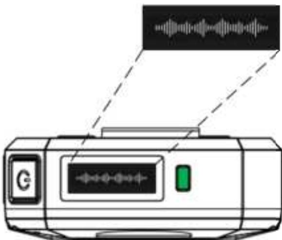
Step 2. When the icon is displayed, say the control word "start recording" within 3 seconds. The BWC will activate the recording according to the command, and the recording icon overlapped with the keyword identification icon is displayed on the LCD (see the following figure).
