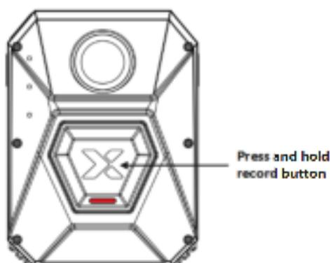
Step 2. Check the BWC LCD. The recording is deactivated and the BWC enters the standby mode in the following scenario: the recording icon and recording status icon disappear and the policeman ID appears, the status light turns from solid red to solid green, and the BWC produces a long prompt tone.
