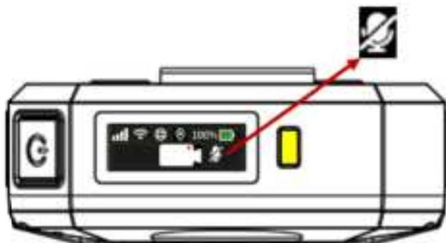
Step 4. To unmute during the recording, repeat step 2 to double-press the FN button. After a short prompt tone is produced and the mute icon is changed to the unmute icon on the LCD (see the following figure), the audio recording is restored.
