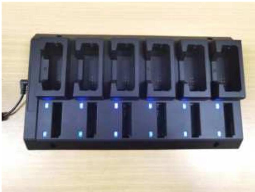
Step 2. Insert the BWC vertically into the Station. The BWC light on the Station turns red, indicating the connection is successful (the light indications are the same as the dock).
