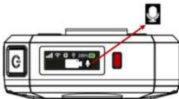
Step 2. Double-press the FN button on the side of the BWC.
