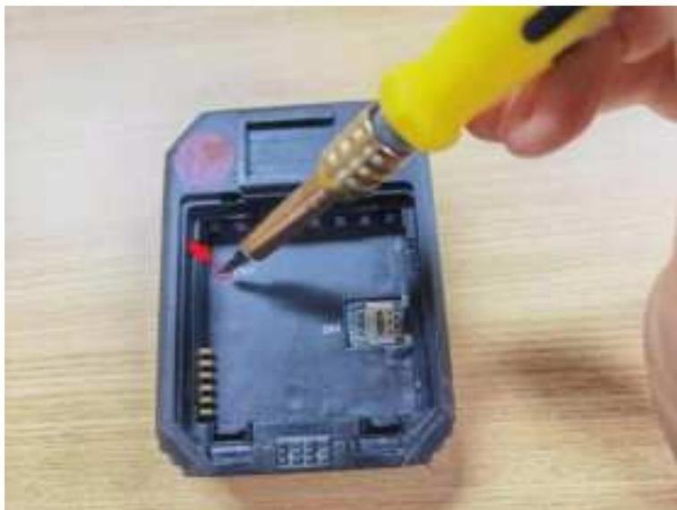
Step 4. After the reset, press the power button to restart the BWC.
