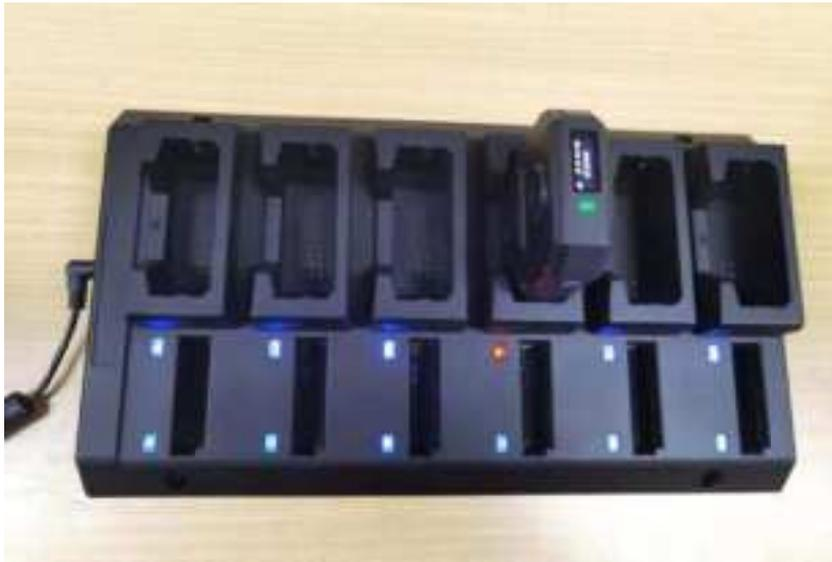
Step 3. Insert the battery into the Station. The battery light of the Station turns red or green. (If the battery is not fully charged yet, the battery light is red. If the battery is fully charged, the battery light is green. The following figure shows that the battery is fully charged and the battery light is green.)
