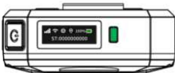
Step 3. In the standby mode, the BWC status and policeman ID are displayed on the LCD (if the BWC is powered on for the first time, no policeman ID is displayed until the ID is configured). On the upper part of the LCD, the status icons for the 4G signal, AP hotspot status, server (platform) connection status, GPS positioning, battery percentage, and battery level are displayed in turn.
