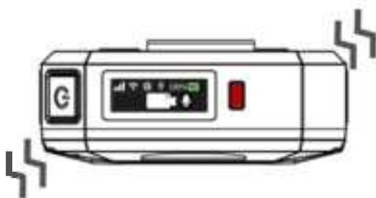
Step 2. After the prompt tone, say the keyword "stop recording" within 3 seconds. The BWC stops recording and returns to the standby mode according to the command. After the operation is successful, the BWC status light turns from red solid to green solid, and the policeman ID is displayed on the LCD (see the following figure).
