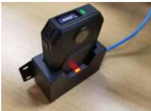
Step 3. If there is video evidence in the BWC needing to be uploaded and synchronized to the platform, the dock can upload the data, and the status bar and upload progress are displayed on the LCD (see the following figure).
