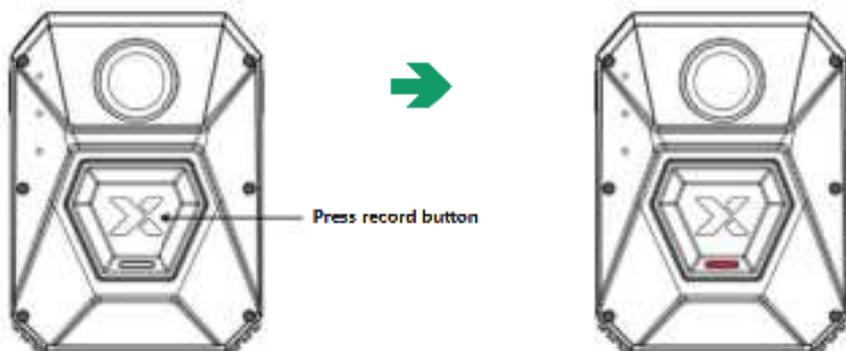
Step 2. When the default recording icon is displayed on the LCD of the BWC (see the following figure) and the BWC produces two short prompt tones, the VigilantEye starts recording.
