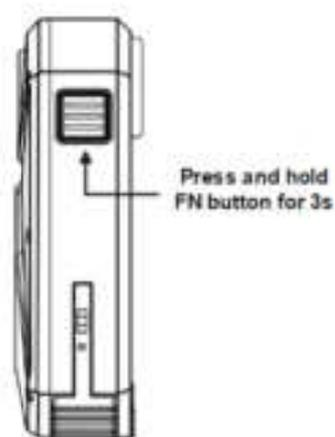
Step 2. The BWC status light turns solid blue, and the AP hotspot is activated (the status light will remain solid blue until the AP hotspot is deactivated or other functions occupy the light indication).
