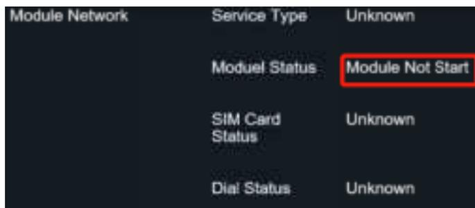
3. The 4G will only work when pull out the BWC from the station. You can check the 4G connection by the LCD:
