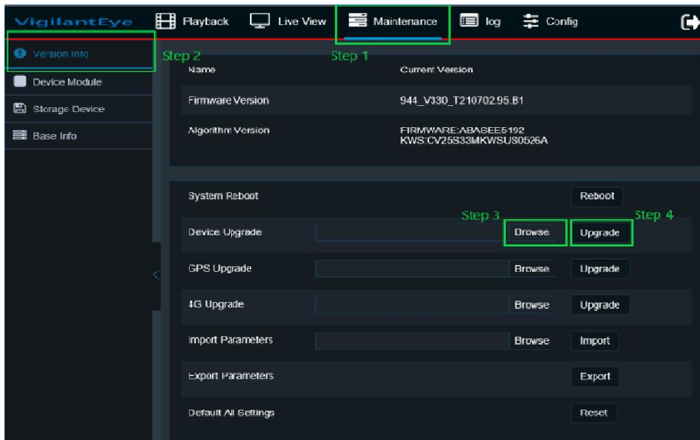
Click **Upgrade** to upgrade the BWC. During the upgrade, do not disconnect the power source from the BWC, which can cause upgrade interruption.
