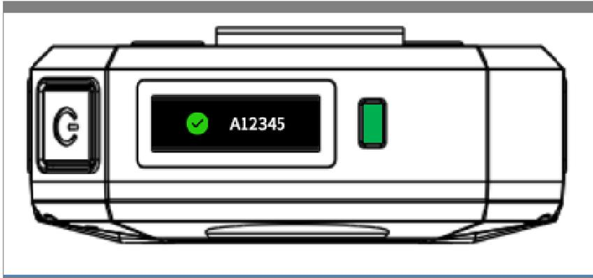
Step 3. The standby status is restored and displayed on the LCD of the BWC after 5 seconds.
