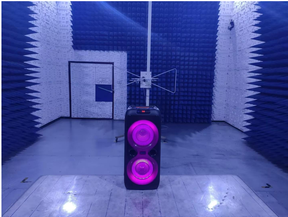
RADIATED EMISSION TEST SETUP ABOVE 1GHz
