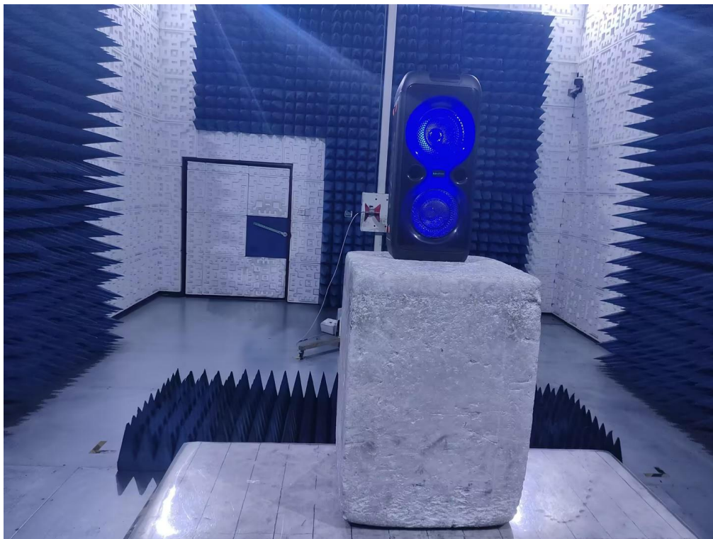
RADIATED EMISSION TEST SETUP ABOVE 1GHz
