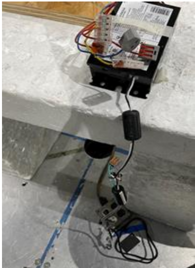
Figure 1.6-1: EUT setup pic with Fair-rite beads.
