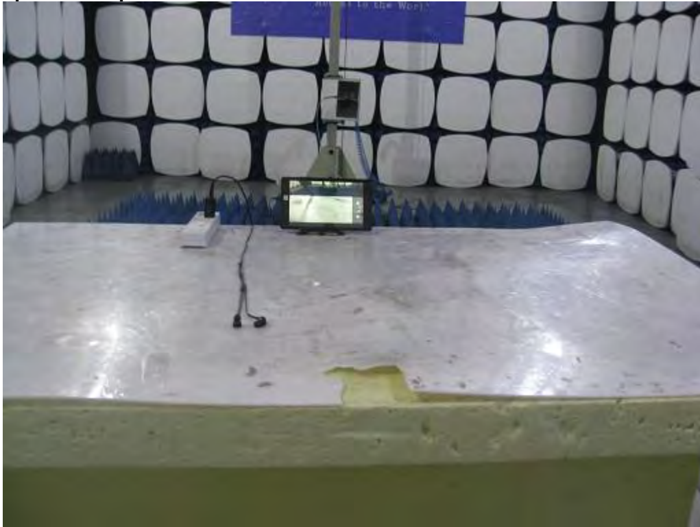
Photograph 3: Set-up for Radiated Emission of above 1GHz
