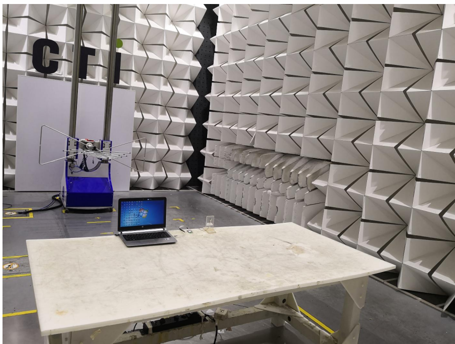
Radiated spurious emission Test Setup-2 (Below 1GHz)
