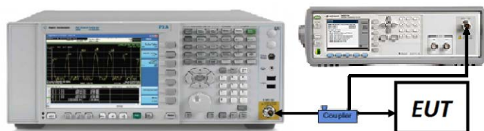
Figure 7-4. Test Instrument & Measurement Setup
