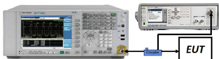
Figure 7-7. Test Instrument & Measurement Setup
