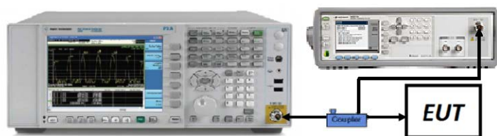
Figure 7-1. Test Instrument & Measurement Setup
