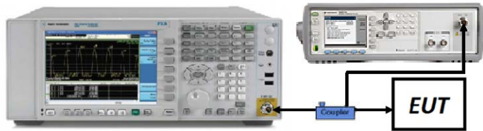
Figure 7-2. Test Instrument & Measurement Setup
