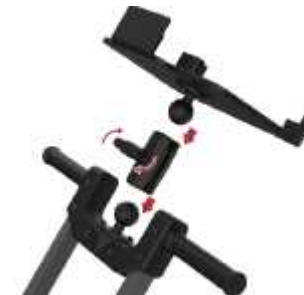
Fig. 19 - How to adjust laptop support
