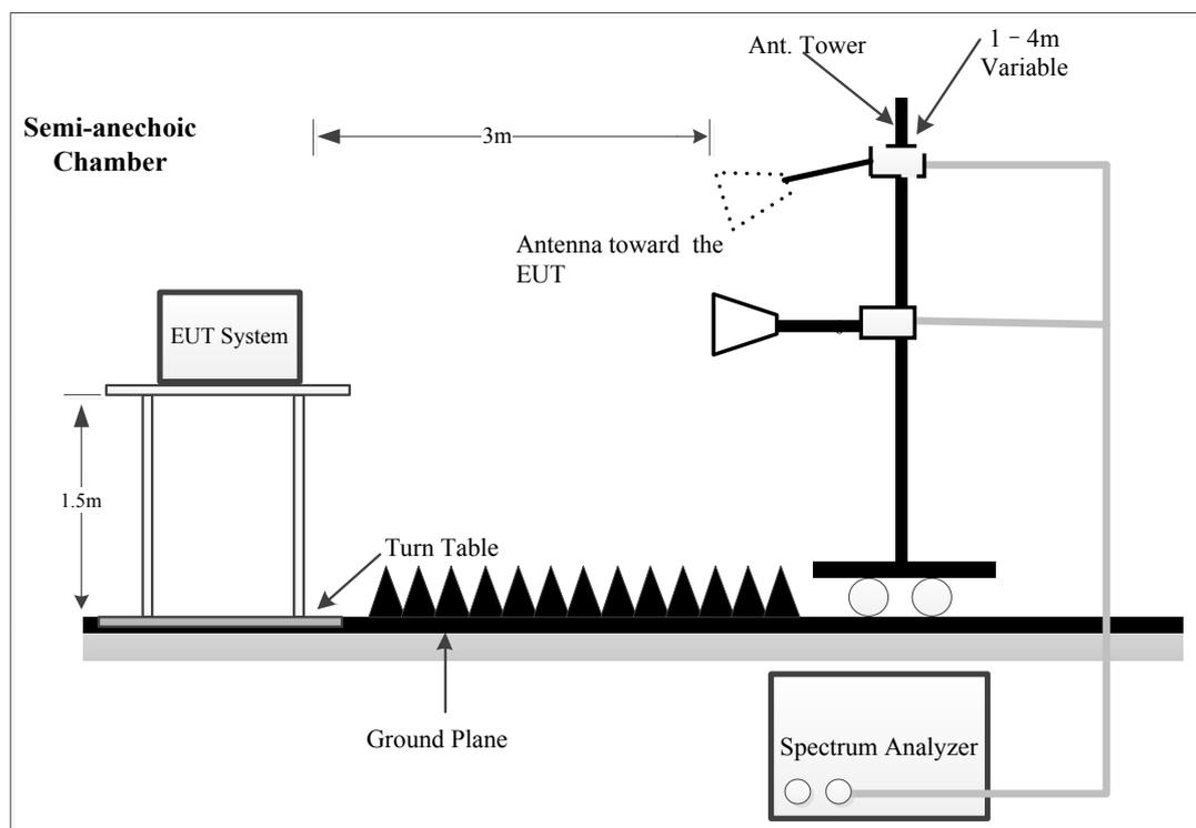
The radiated emissions were performed in the 3 meters distance, using the setup accordance with the ANSI C63.10-2013. The specification used was the FCC 15.209, and FCC 15.247, RSS-247, RSS-Gen limits.
