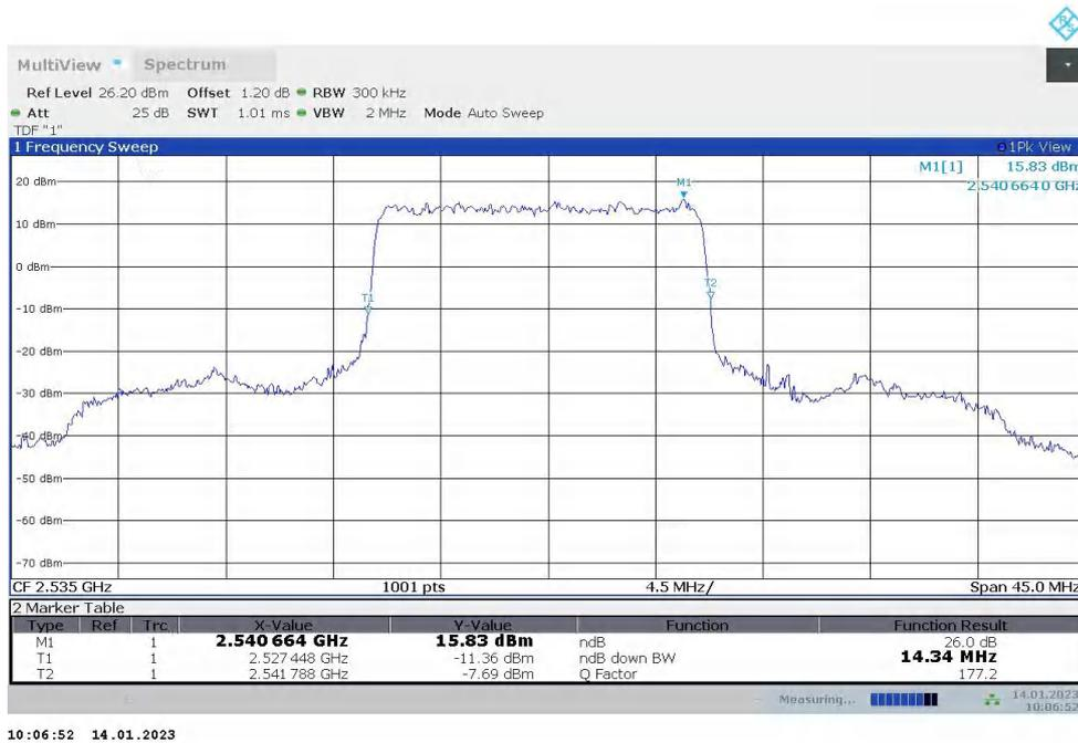
n7,15MHz Bandwidth,DFT-s-QPSK (-26dBc BW)
