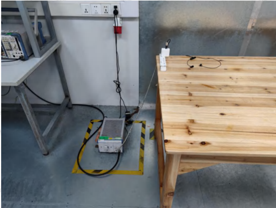
Photo of Power Line Conducted Emission Test
