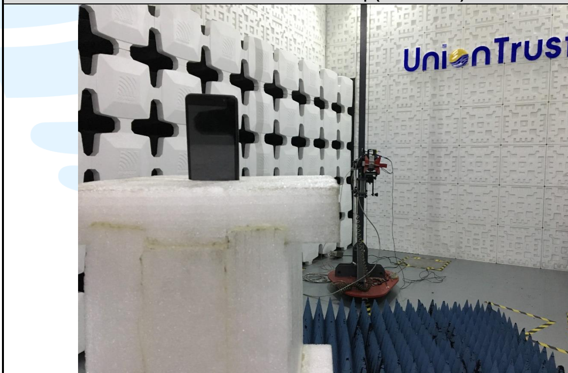
Radiated emission Test Setup (Above 1 GHz)
