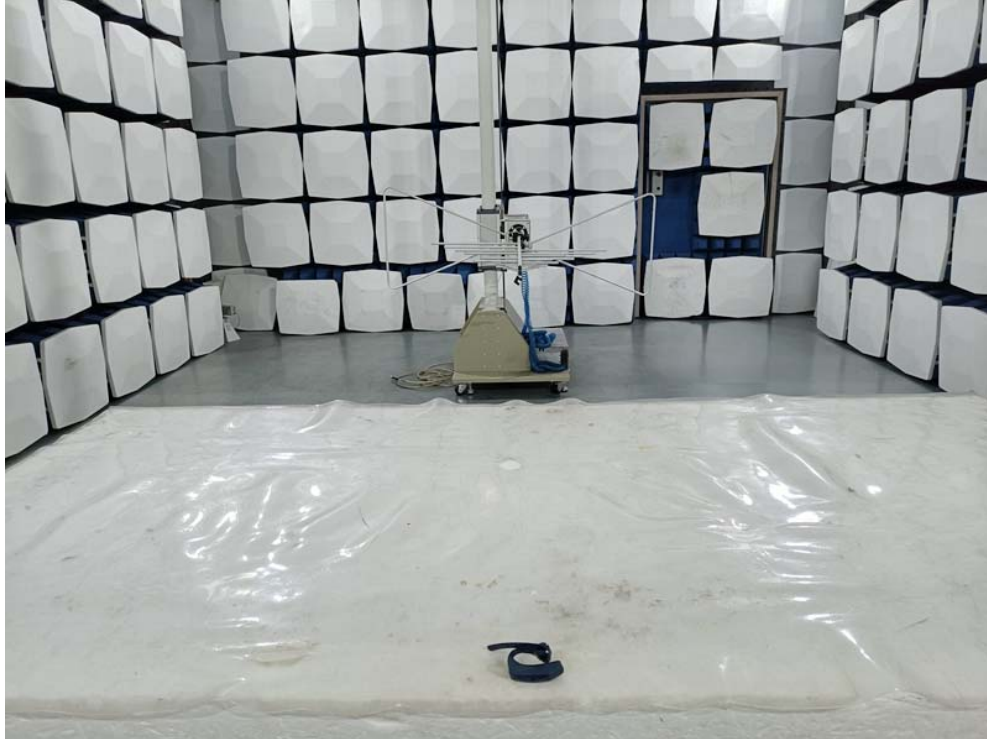
Radiated Emission Test Setup:
