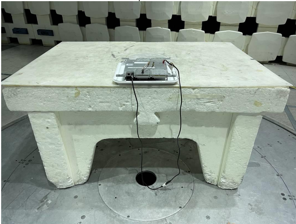
Radiated Emissions Test Setup From 30 MHz-1000 MHz – Photo 1
