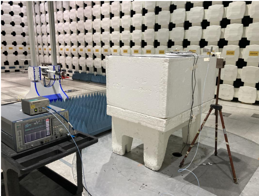
Radiated Emissions Test Setup From 18-20 GHz – Photo 1
