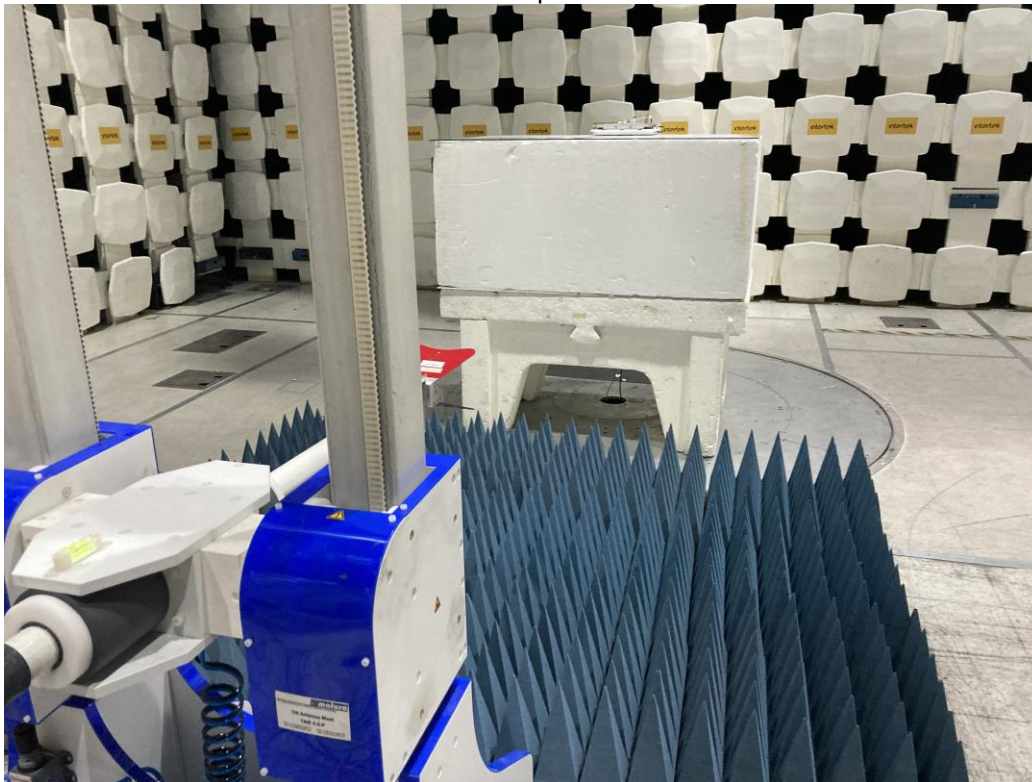
Radiated Emissions Test Setup From 1-18 GHz – Photo 1
