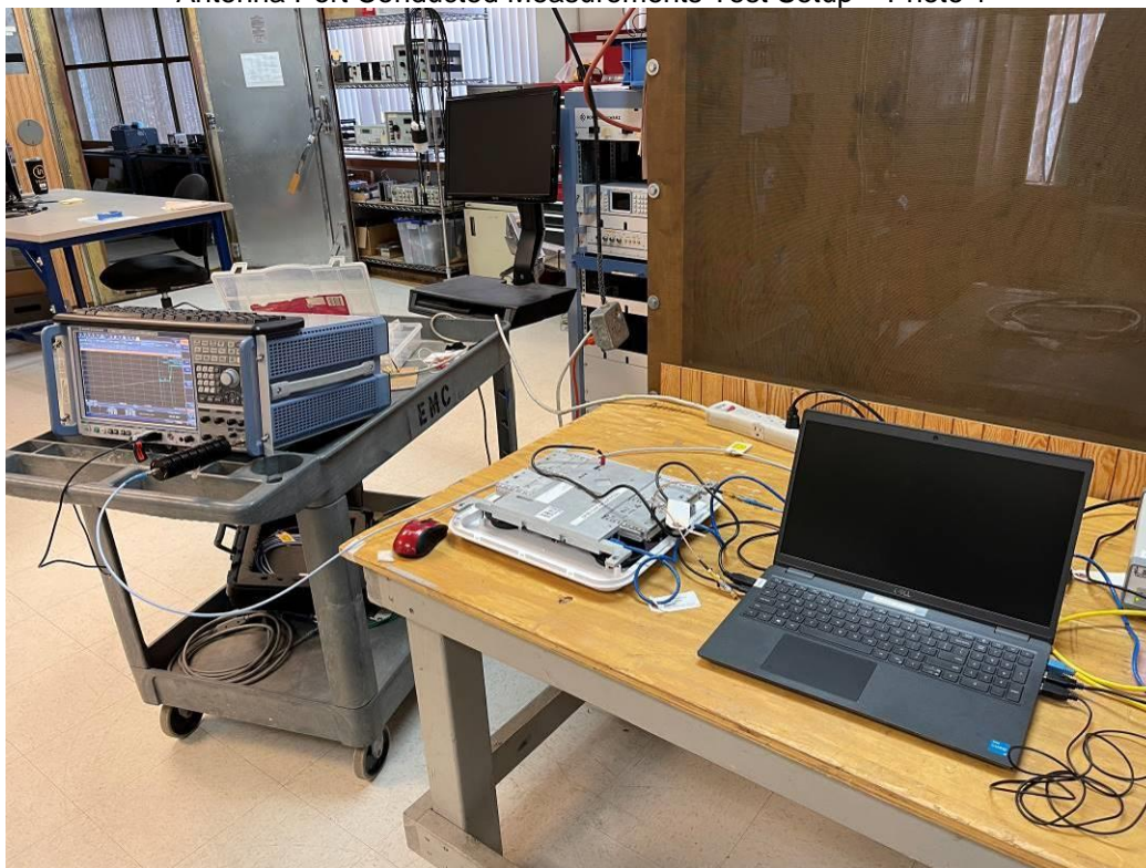
Radiated Emissions Test Setup From 9 kHz-30 MHz – Photo 1
