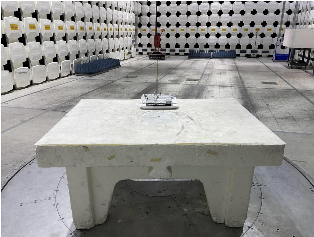
Radiated Emissions Test Setup From 1-18 GHz – Photo 1
