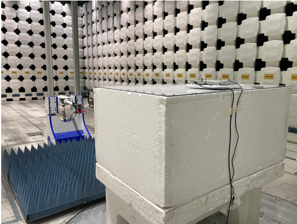
Radiated Emissions Test Setup From 18-20 GHz – Photo 1
