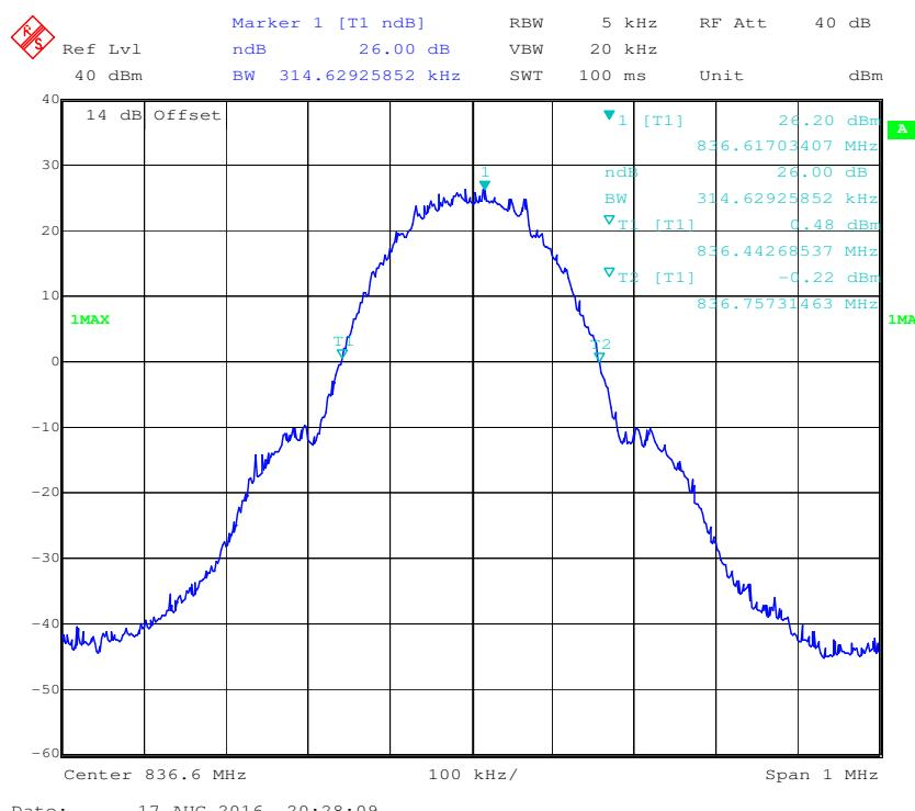
**PCS Band (Part 24E)****99% Occupied Bandwidth for GSM (GMSK) Mode**
