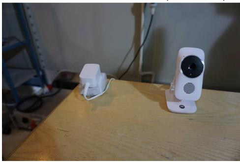
Radiated Emissions (30MHz-1GHz) Test Setup
