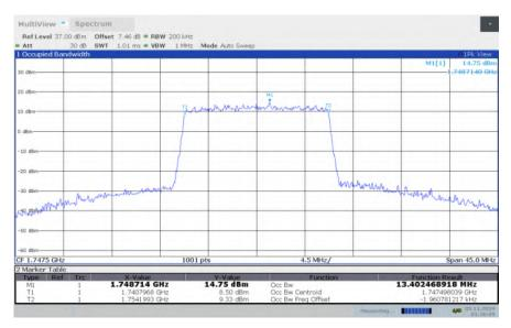
LTE band 4, 15MHz Bandwidth, HIGH, 64QAM (99% BW)
