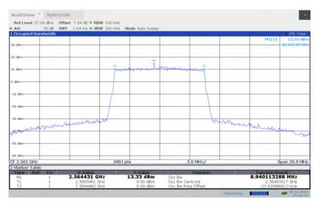
LTE band 7, 10MHz Bandwidth, HIGH, 64QAM (99% BW)
