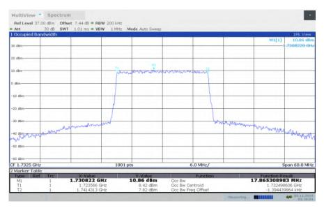
LTE band 4 , 20MHz Bandwidth, HIGH, QPSK (99% BW)
