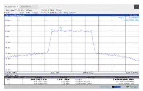
LTE band 5, 3MHz Bandwidth, HIGH, 64QAM (99% BW)
