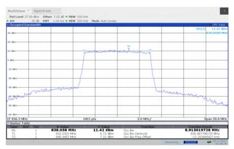
LTE band 5, 10MHz Bandwidth, HIGH, QPSK (99% BW)
