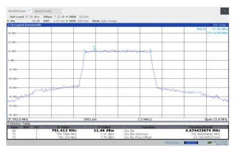
LTE band 14, 5MHz Bandwidth, HIGH, QPSK (99% BW)
