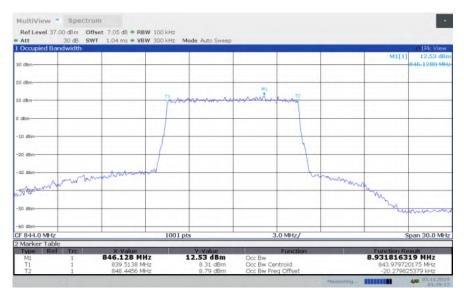
LTE band 5, 10MHz Bandwidth, HIGH, 64QAM (99% BW)
