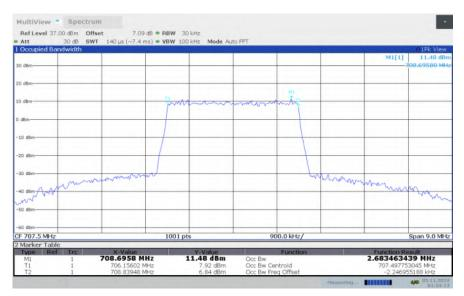
LTE band 12, 3MHz Bandwidth, HIGH, QPSK (99% BW)
