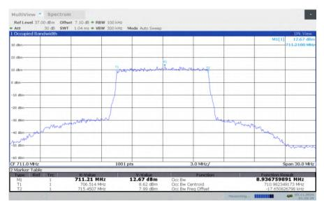
LTE band 12, 10MHz Bandwidth, HIGH, 64QAM (99% BW)
