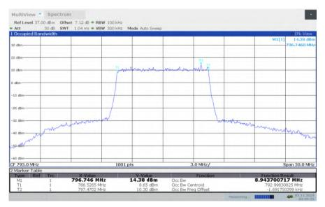
LTE band 14, 10MHz Bandwidth, HIGH, 64QAM (99% BW)
