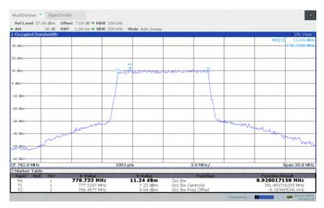
LTE band 13, 10MHz Bandwidth, HIGH, QPSK (99% BW)
