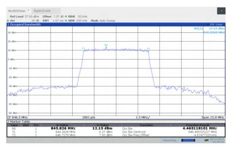
LTE band 5, 5MHz Bandwidth, HIGH, 64QAM (99% BW)
