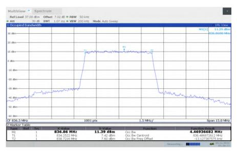
LTE band 5, 5MHz Bandwidth, HIGH, QPSK (99% BW)
