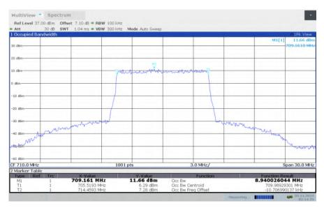
LTE band 17, 10MHz Bandwidth, HIGH, QPSK (99% BW)
