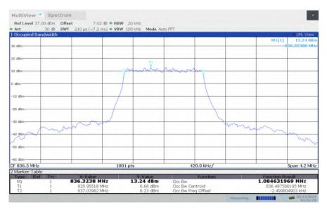
LTE band 5 , 1.4MHz Bandwidth, HIGH, QPSK (99% BW)
