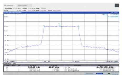
LTE band 12, 5MHz Bandwidth, HIGH, QPSK (99% BW)
