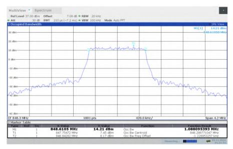
LTE band 5, 1.4MHz Bandwidth, HIGH, 64QAM (99% BW)
