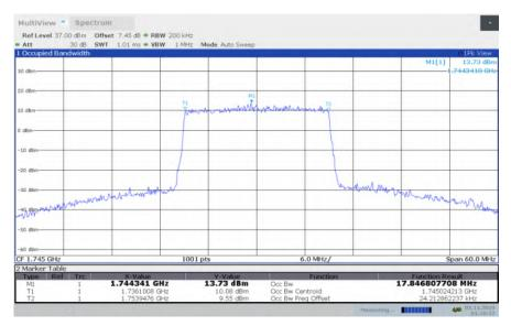
LTE band 4, 20MHz Bandwidth, HIGH, 64QAM (99% BW)
