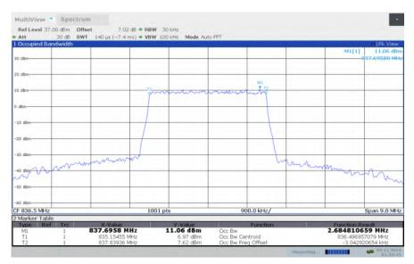
LTE band 5, 3MHz Bandwidth, HIGH, QPSK (99% BW)
