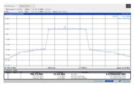
LTE band 13, 5MHz Bandwidth, HIGH, QPSK (99% BW)
