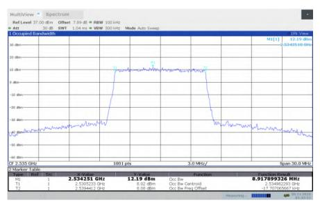
LTE band 7, 10MHz Bandwidth, HIGH, QPSK (99% BW)
