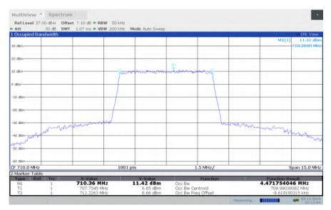
LTE band 17, 5MHz Bandwidth, HIGH, QPSK (99% BW)
