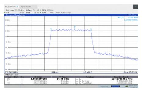
LTE band 7, 15MHz Bandwidth, HIGH, 64QAM (99% BW)
