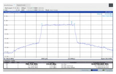
LTE band 13, 10MHz Bandwidth, HIGH, 64QAM (99% BW)
