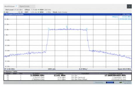
LTE band 7, 20MHz Bandwidth, HIGH, 64QAM (99% BW)
