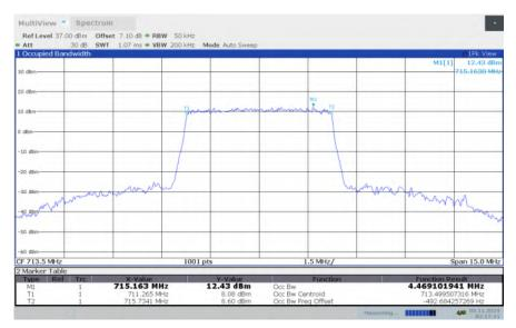
LTE band 17, 5MHz Bandwidth, HIGH, 64QAM (99% BW)
