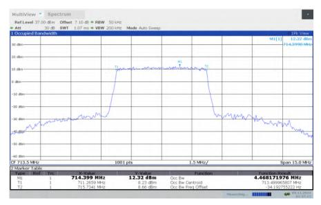
LTE band 12, 5MHz Bandwidth, HIGH, 64QAM (99% BW)
