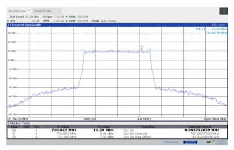
LTE band 12, 10MHz Bandwidth, HIGH, QPSK (99% BW)
