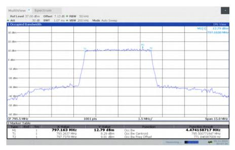
LTE band 14, 5MHz Bandwidth, HIGH, 64QAM (99% BW)
