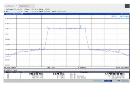
LTE band 13, 5MHz Bandwidth, HIGH, 64QAM (99% BW)
