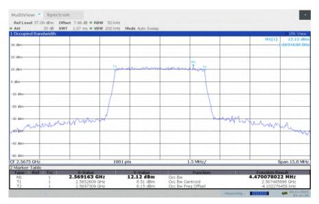
LTE band 7, 5MHz Bandwidth, HIGH, 64QAM (99% BW)
