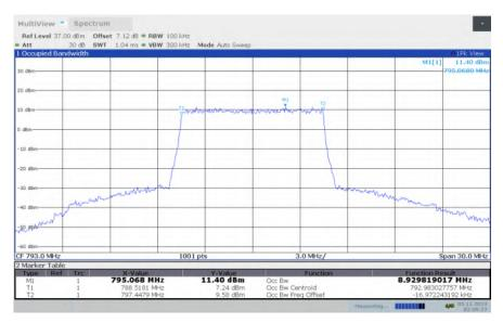
LTE band 14, 10MHz Bandwidth, HIGH, QPSK (99% BW)
