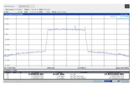
LTE band 7, 20MHz Bandwidth, HIGH, QPSK (99% BW)
