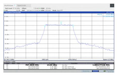
LTE band 12 , 1.4MHz Bandwidth, HIGH, QPSK (99% BW)
