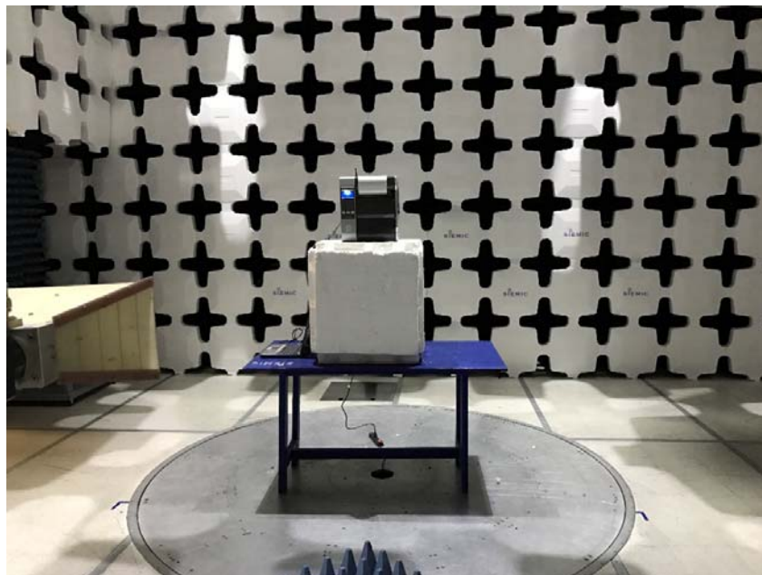
Radiated Emissions (>1GHz) – Front View
