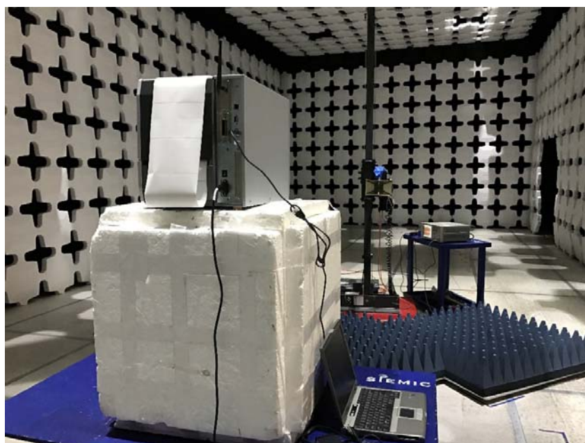
Radiated Emissions (>1GHz) – Rear View
