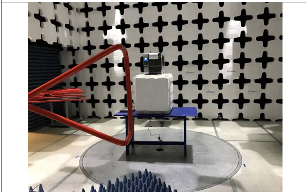
Radiated Emissions (<1GHz) – Rear View
