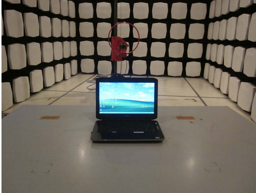
Measurement of Radiated Emission Test Set Up
