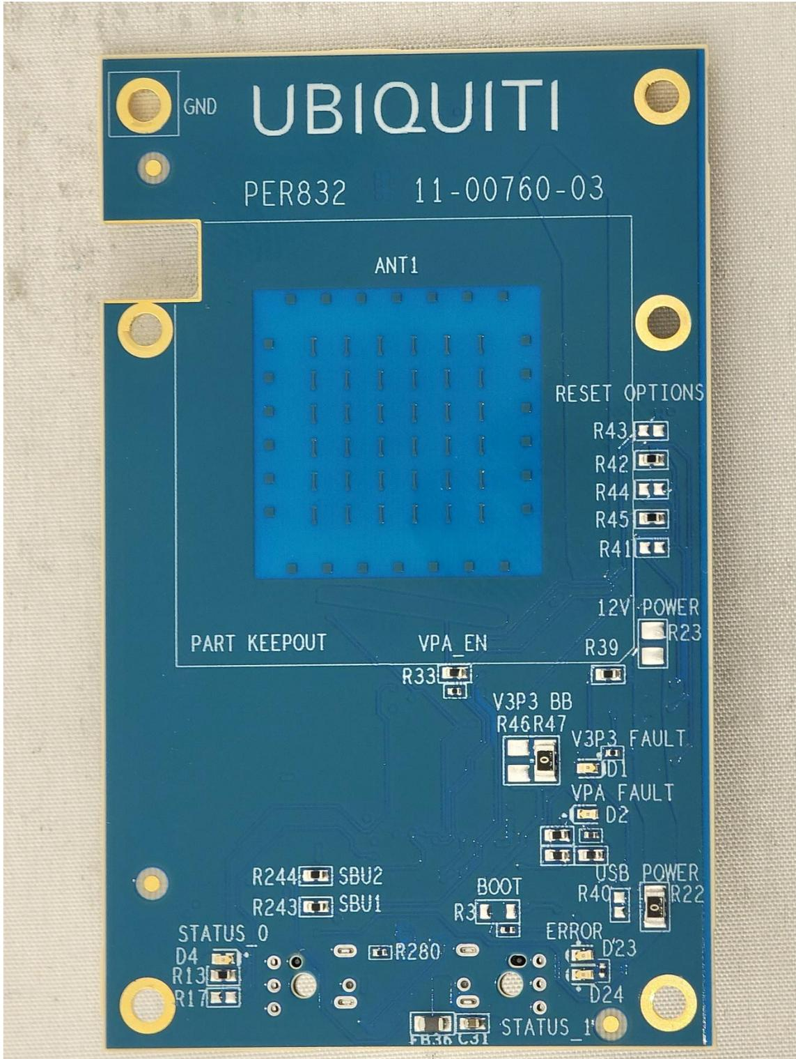
**Photograph 10: Front View of the 60GHz Antenna PCB**
