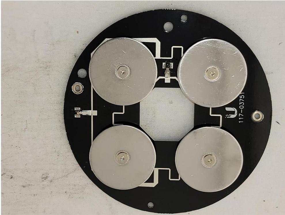
**Photograph 8: Front View of the 5GHz Antenna**
