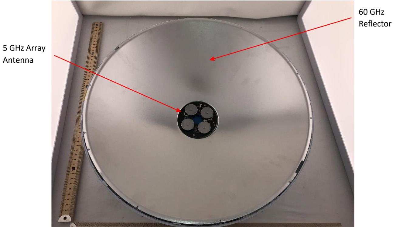
**Photograph 1: Front View of DUT With Reflector**
