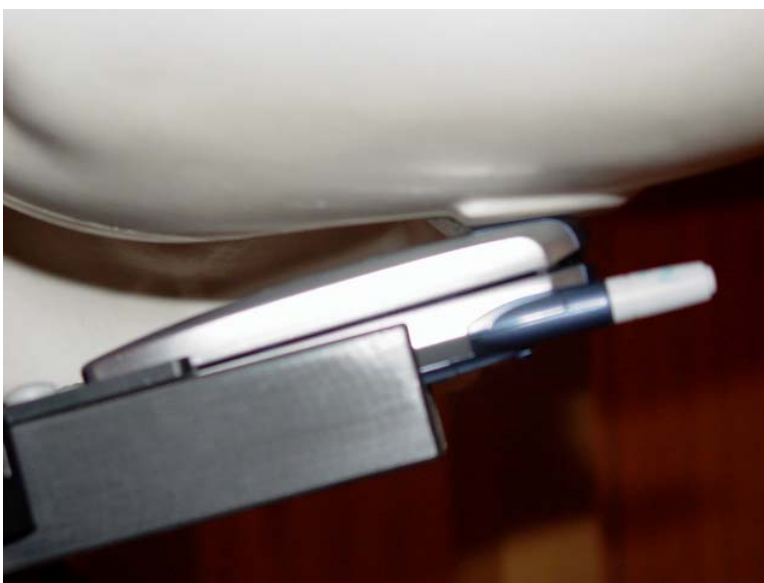
Figure 10.3 phone against the head (right tilt position, swivel closed, antenna retracted)
