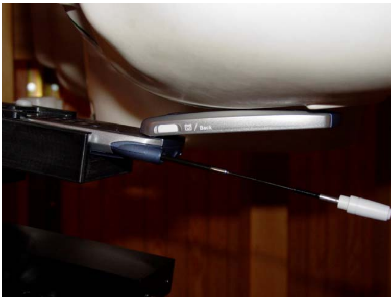
Figure 10.8 phone against the head (right cheek position, swivel open, antenna extended)
