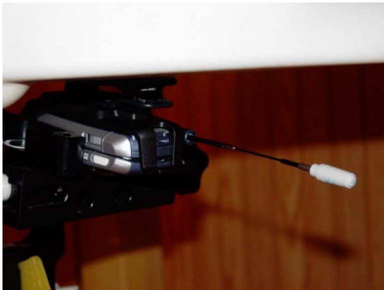
Figure 10.11 body SAR setup (with holster, swivel closed, antenna extended)
