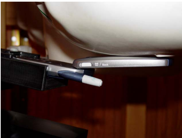
Figure 10.6 phone against the head (right cheek position, swivel open, antenna retracted)
