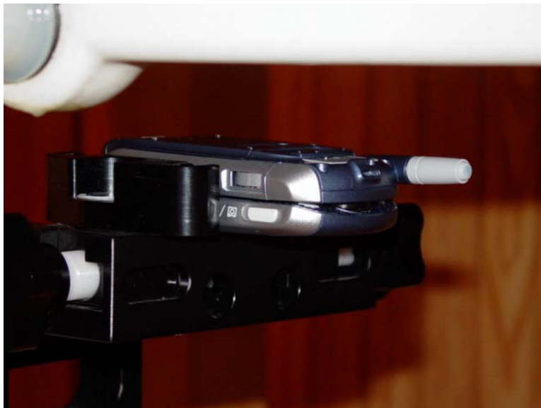
Figure 10.14 body SAR setup (with 25mm air separation, swivel closed, antenna retracted)
