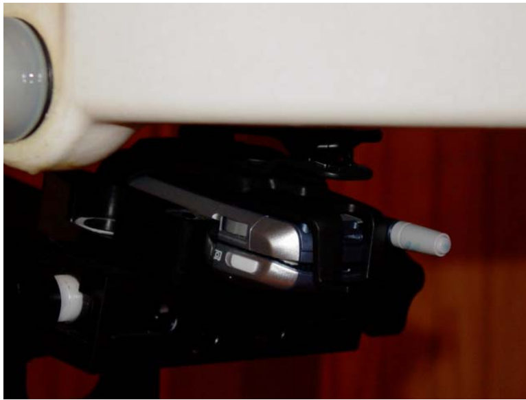
Figure 10.10 body SAR setup (with holster, swivel closed, antenna retracted)
