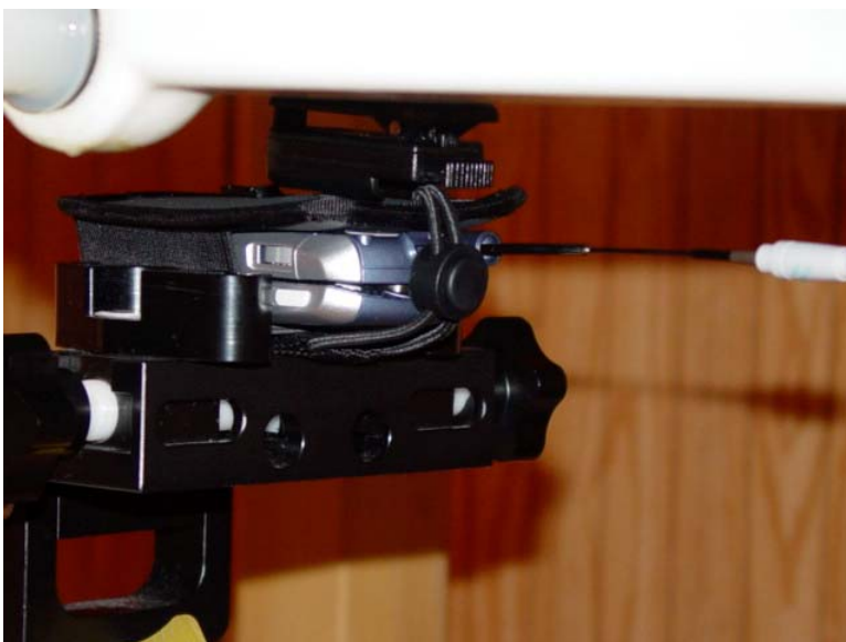
Figure 10.13 body SAR setup (with leather case, swivel closed, antenna extended)
