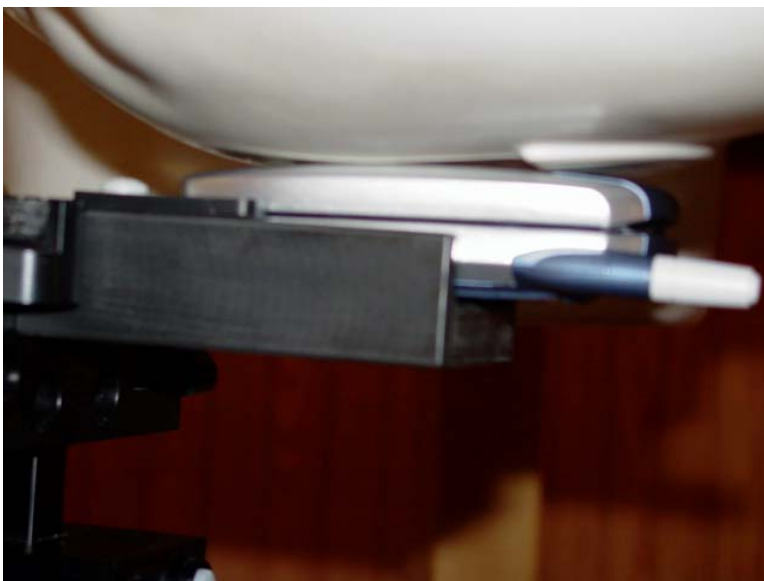
Figure 10.2 phone against the head (right cheek position, swivel closed, antenna retracted)
