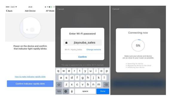
While under AP mode, press the button" Confirm indicator slowly blink", and input the WiFi password to complete the connecting.
