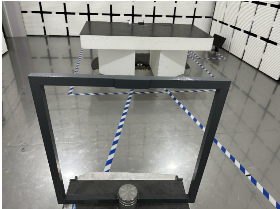
Radiation Emission Test Setup (Below 30MHz)
