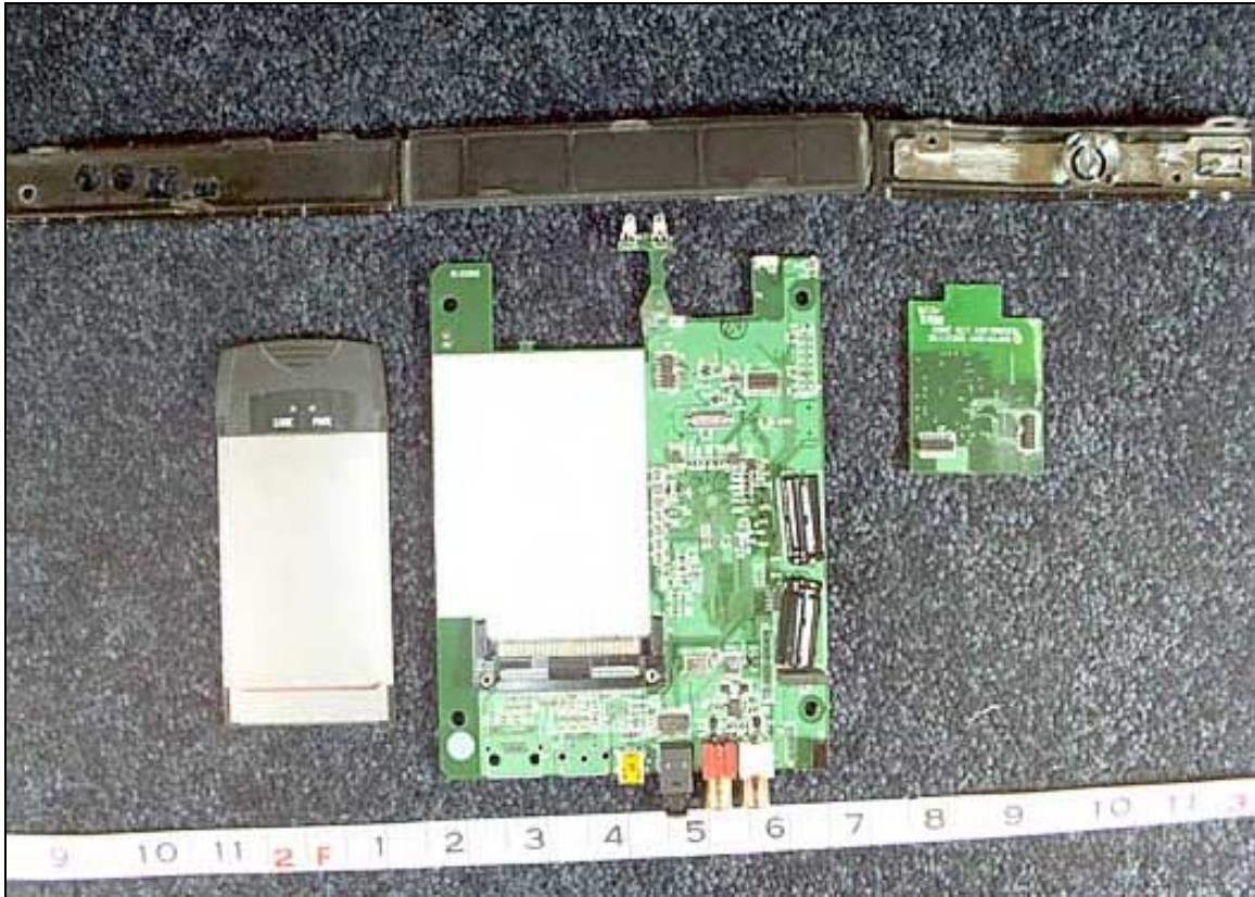
Base Sides, 2.4 GHz Transmitter and 900 MHz Transmitter Removed
