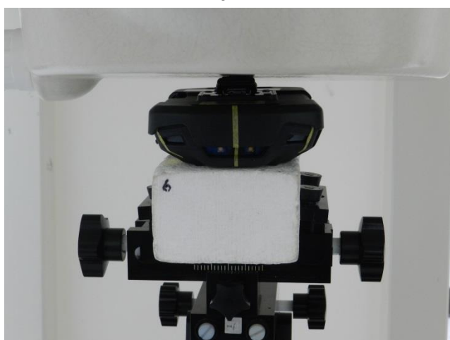
Front with Rigid Holster, Test Separation 0 mm
