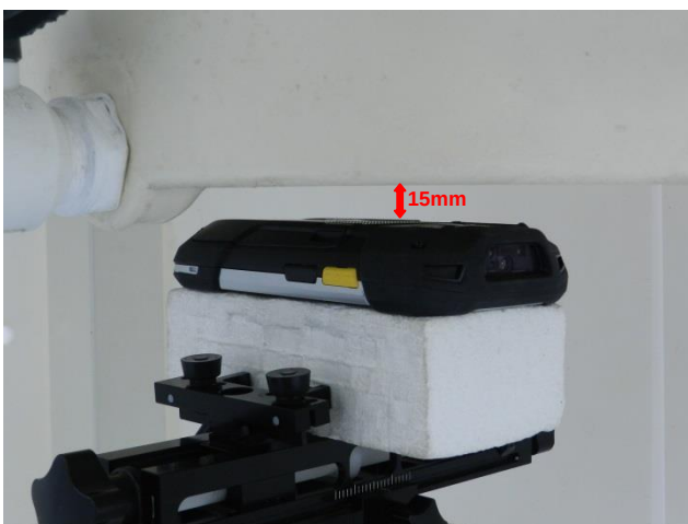
Back , Test Separation 15 mm
