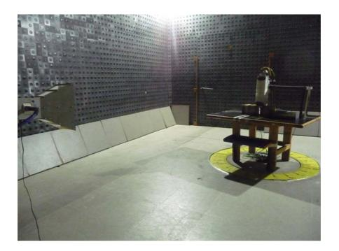
$\label{eq:Photograph No.6} Photograph No.6 \\ Spurious emissions measurement setup in the anechoic chamber in 18 – 27 GHz$
