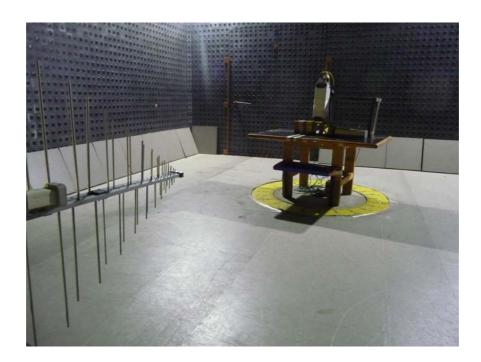
$\label{eq:Photograph No.5} Photograph No.5 \\ Spurious emissions measurement setup in the anechoic chamber in 1 – 18 GHz$
