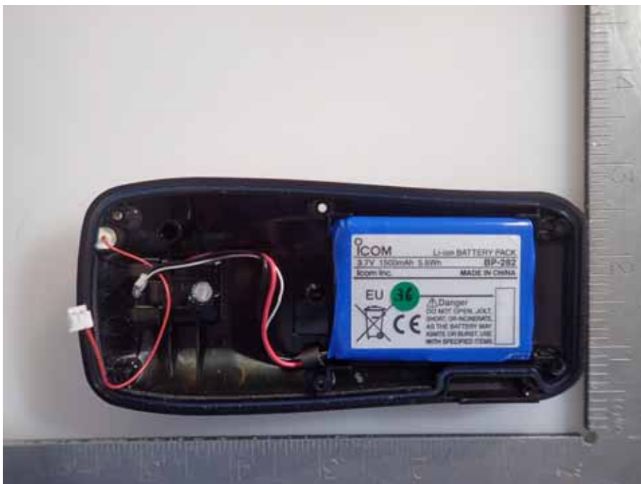
Li-ion Chargeable Battery (M/N: BP-282, 3.7V, 1500mAh)
