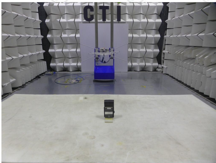
Radiated spurious emission Test Setup-2(30MHz-1GHz)
