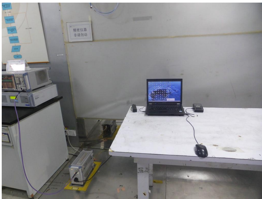
Conducted Emissions Test Setup
