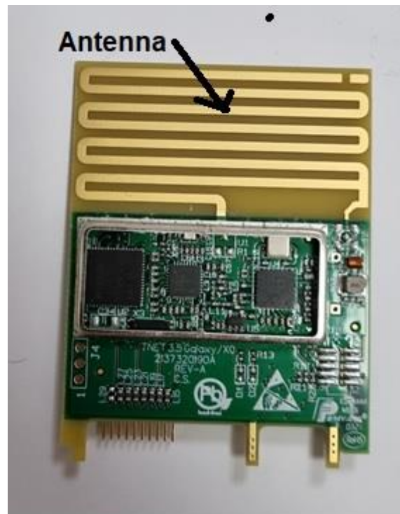
RF Card (TNET3.5) shield removed- top view
