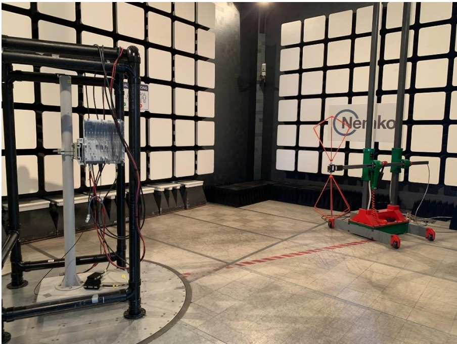
Figure 3.5-2: EUT Set-up photo for Radiated Compliance Testing
