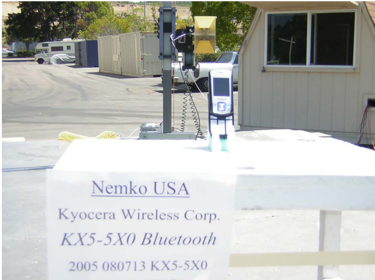
Photograph 5. Fundamental Radiated Emissions Test Configuration (Open)
