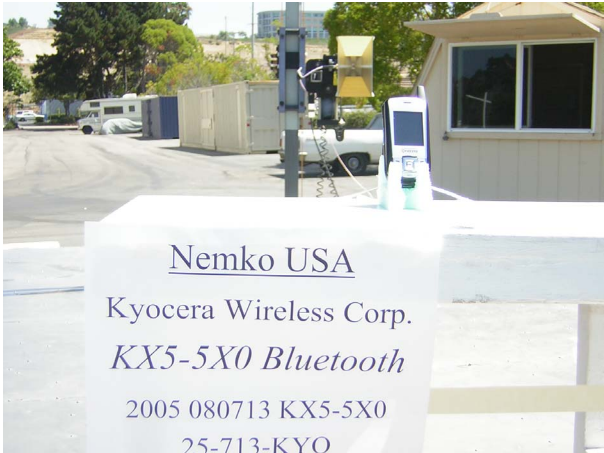
Photograph 6. Fundamental Radiated Emissions Test Configuration (Closed)
