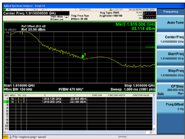
Band25 / 15MHz / High CH / QPSK / 1 RB
