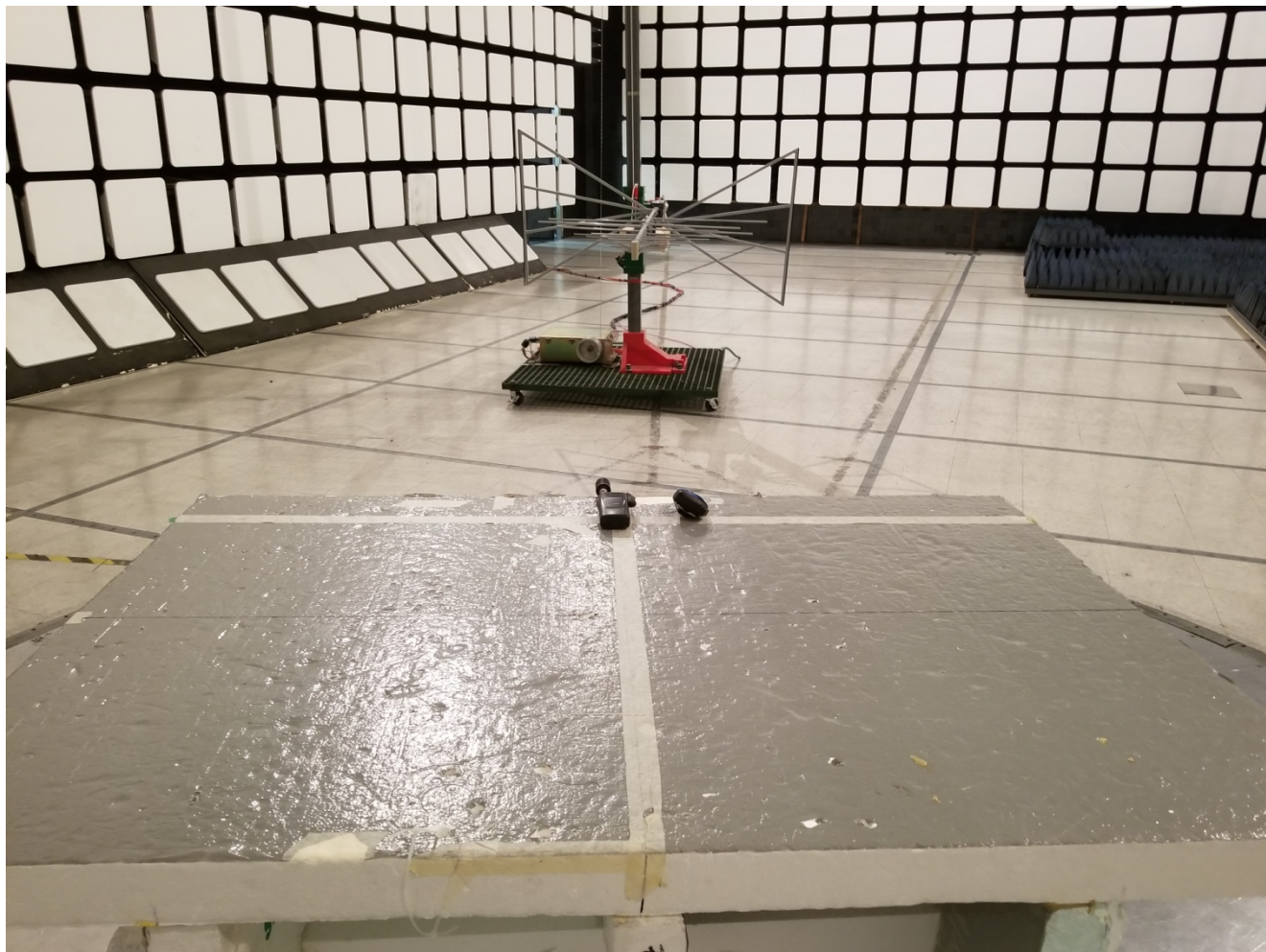
Radiated Emissions at 3 m, 30 - 1000 MHz Orthogonal Position 1
