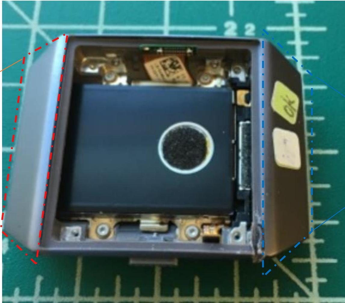
GPS antenna molded to the housing
