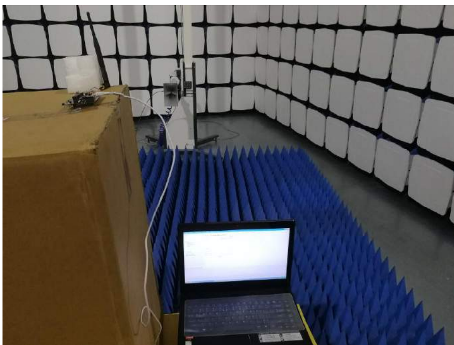
Test Mode_2 - Radiated Emission test view (Frequency above 1GHz)
