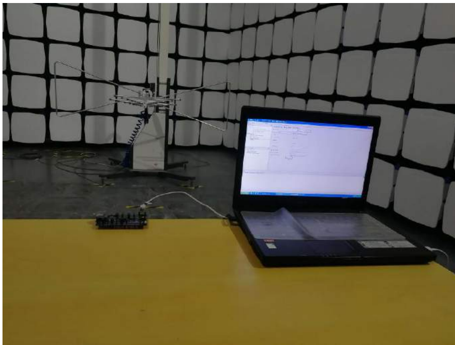
Test Mode_3 - Radiated Emission test view (Frequency above 1GHz)
