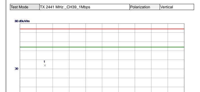
Reading Correct Measure No. Freq. Limit Margin Level Factor ment dB MHz dBuV/m dBuV/m dBuV/mdB Detector Comment 1 \* 4882.0000 50.83 -16. 97 33.86 74.00 -40. 14 Peak
