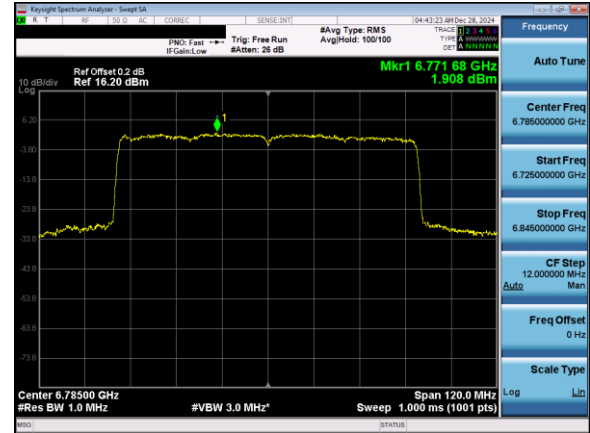
Plot 7-190. Power Spectral Density Plot CDD Primary Antenna 3b (80MHz 802.11ax (UNII Band 7) – Ch. 167)
