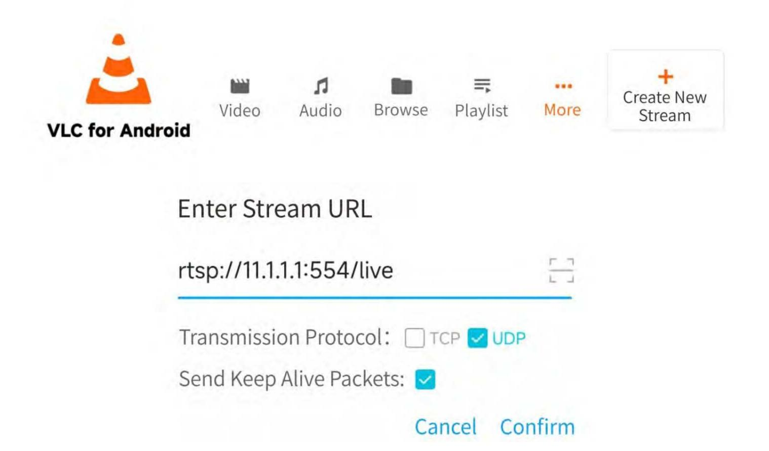
Enter the address and click "Connect" to observe the real-time image on the mobile device.
