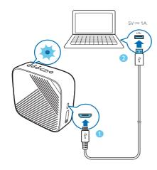
Connect the USB cable between the micro-USB socket on the speaker and a USB socket on your computer or a charger.
