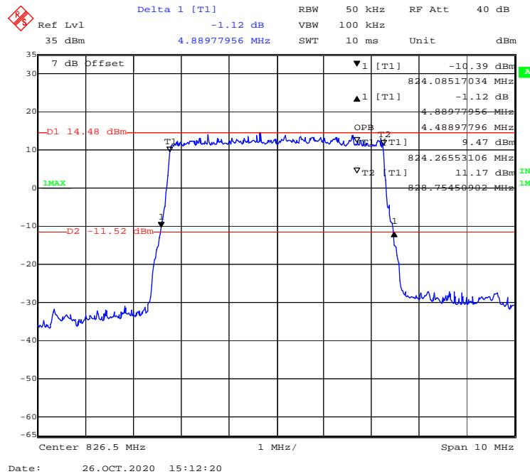
**QPSK (10.0 MHz) - 99% Occupied & 26 dB Emissions Bandwidth, Low channel**
