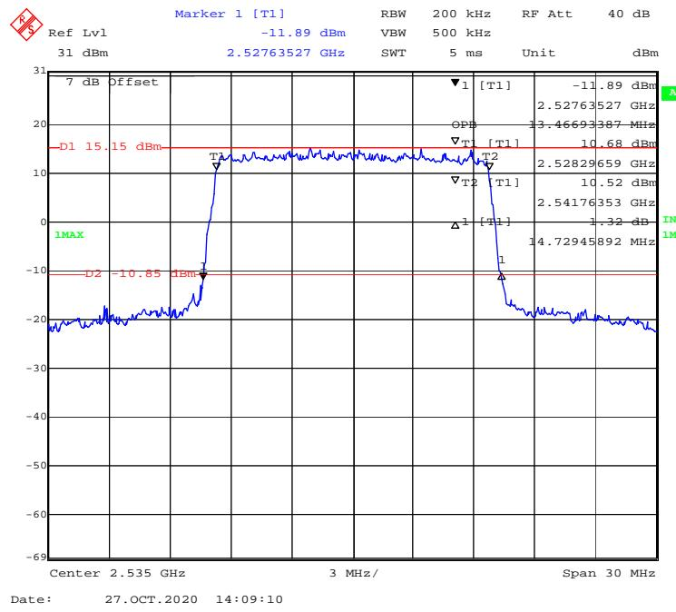
**QPSK (20 MHz) - 99% Occupied & 26 dB Emissions Bandwidth, Middle channel**
