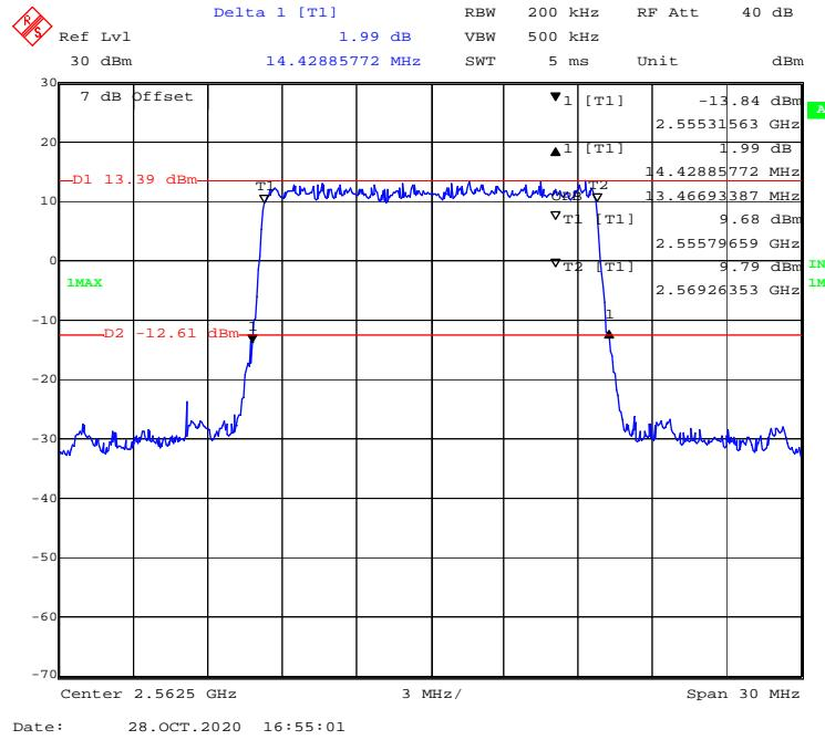
**QPSK (20 MHz) - 99% Occupied & 26 dB Emissions Bandwidth, Low channel**
