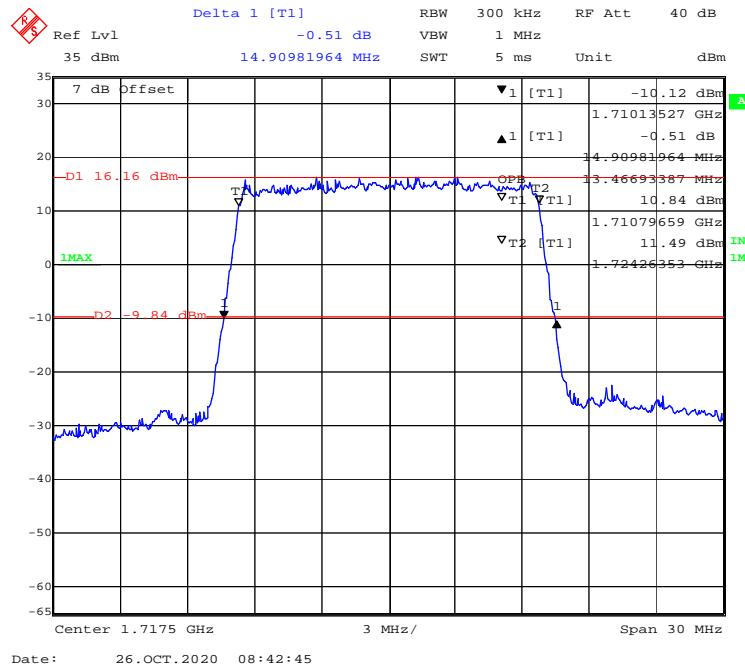
**16-QAM (20 MHz) - 99% Occupied & 26 dB Emissions Bandwidth, Low channel**
