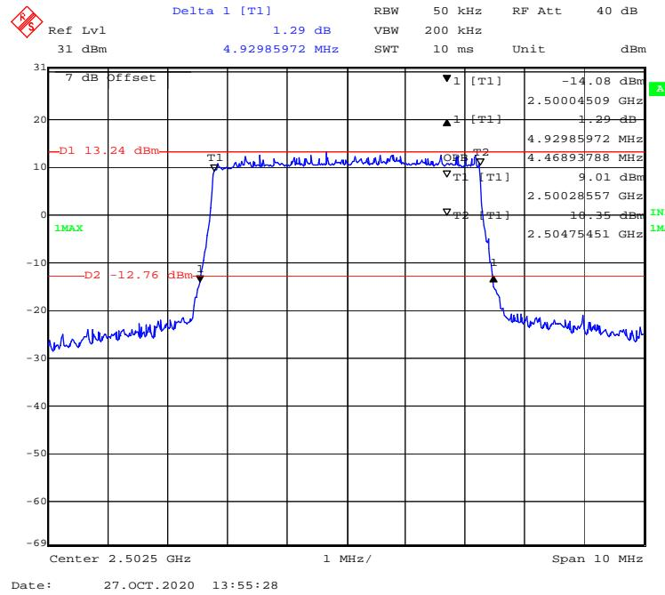
**16-QAM (10 MHz) - 99% Occupied & 26 dB Emissions Bandwidth, Low channel**
