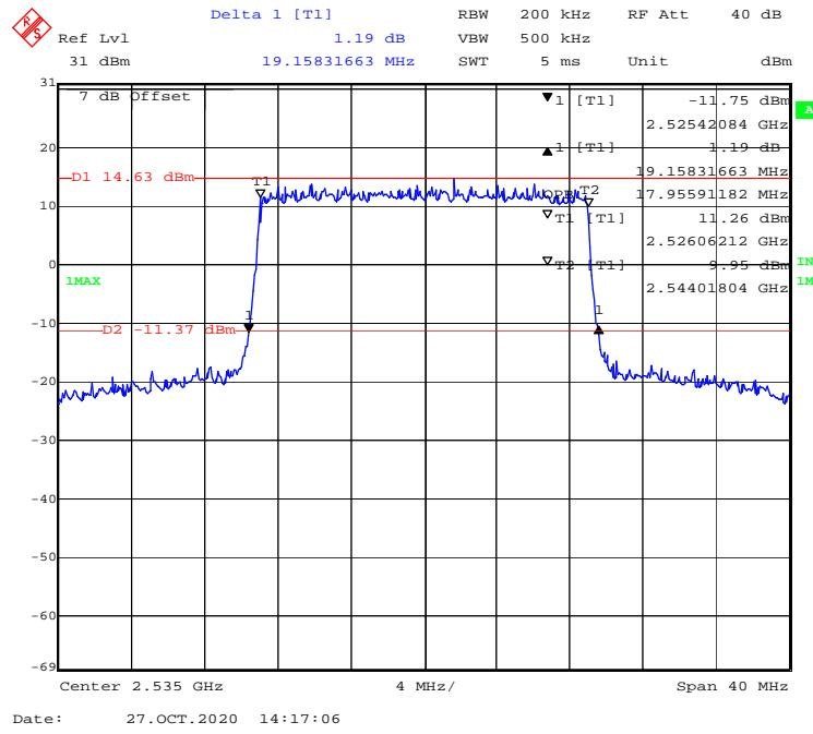
**QPSK (5 MHz) - 99% Occupied & 26 dB Emissions Bandwidth, High channel**
