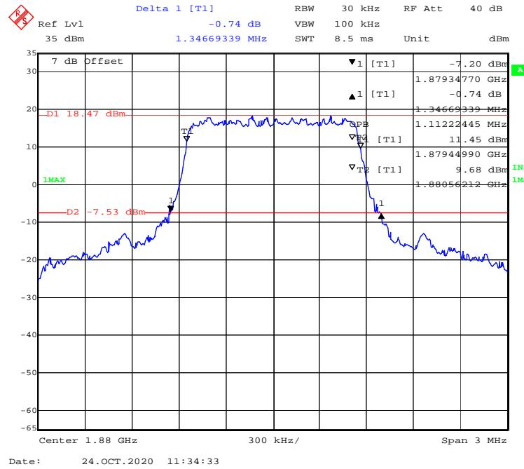
**16-QAM (3 MHz) - 99% Occupied & 26 dB Emissions Bandwidth, Middle channel**
