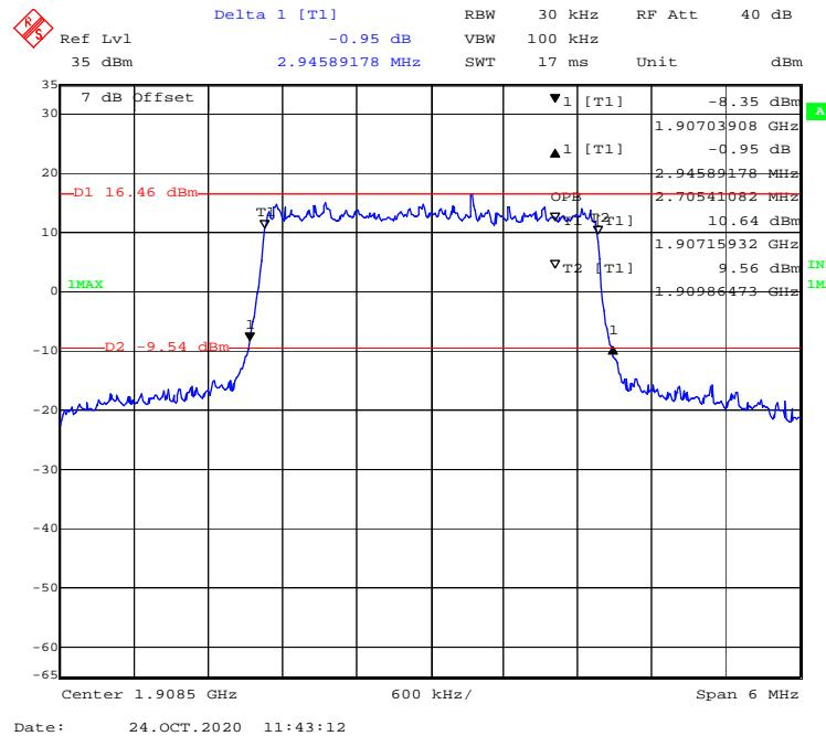
**16-QAM (5 MHz) - 99% Occupied & 26 dB Emissions Bandwidth, High channel**
