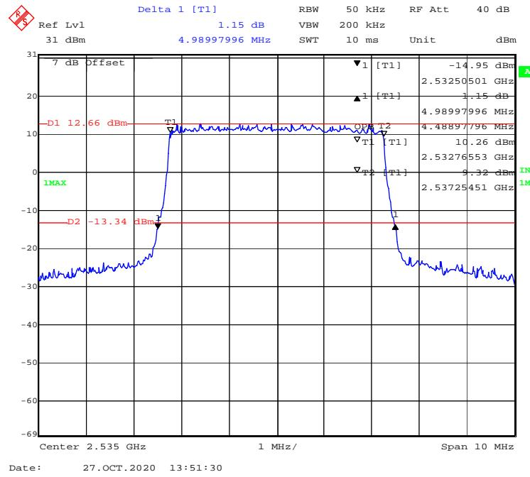
**QPSK (10 MHz) - 99% Occupied & 26 dB Emissions Bandwidth, Middle channel**
