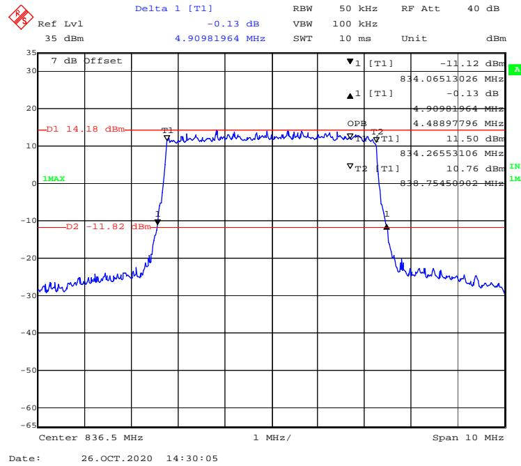
**16-QAM (10.0 MHz) - 99% Occupied & 26 dB Emissions Bandwidth, Middle channel**
