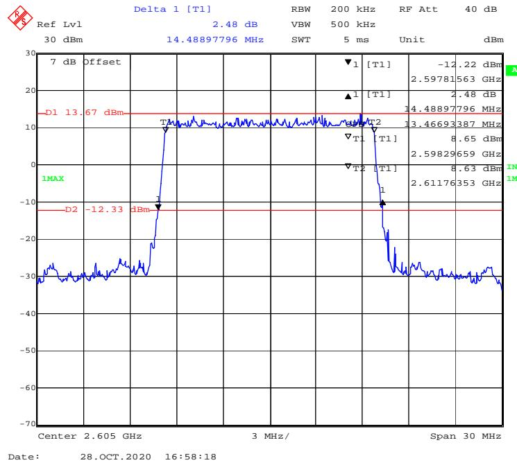
**16-QAM (20 MHz) - 99% Occupied & 26 dB Emissions Bandwidth, Middle channel**
