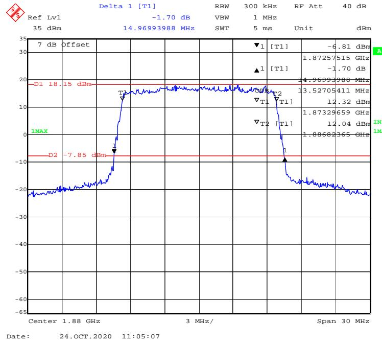
**16-QAM (20 MHz) - 99% Occupied & 26 dB Emissions Bandwidth, Middle channel**
