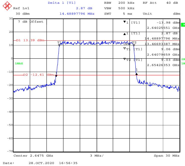
**16-QAM (20 MHz) - 99% Occupied & 26 dB Emissions Bandwidth, High channel**
