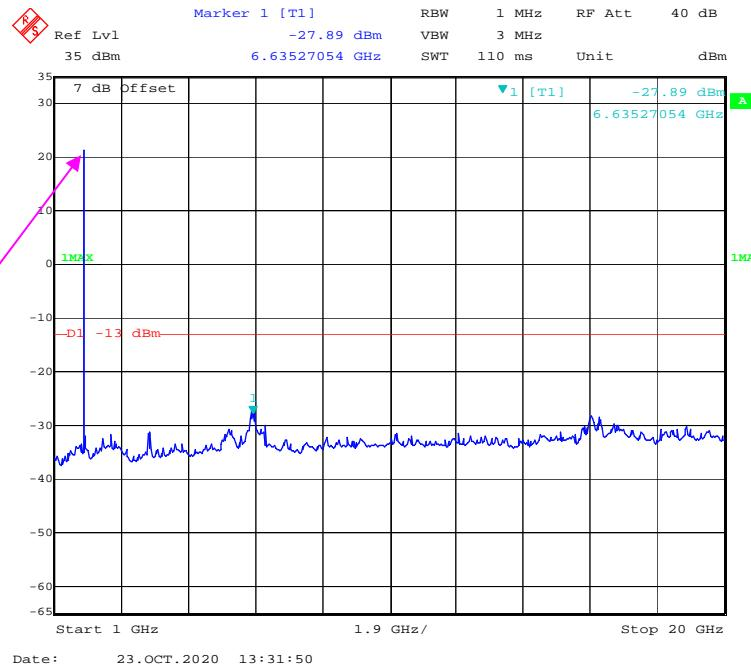
**30 MHz – 1GHz WCDMA (HSDPA) Mode , Low channel**
