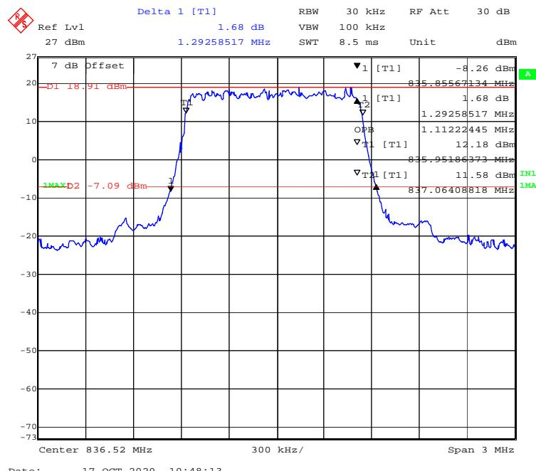
**EVDO mode, 99% Occupied & 26 dB Emissions Bandwidth High channel**
