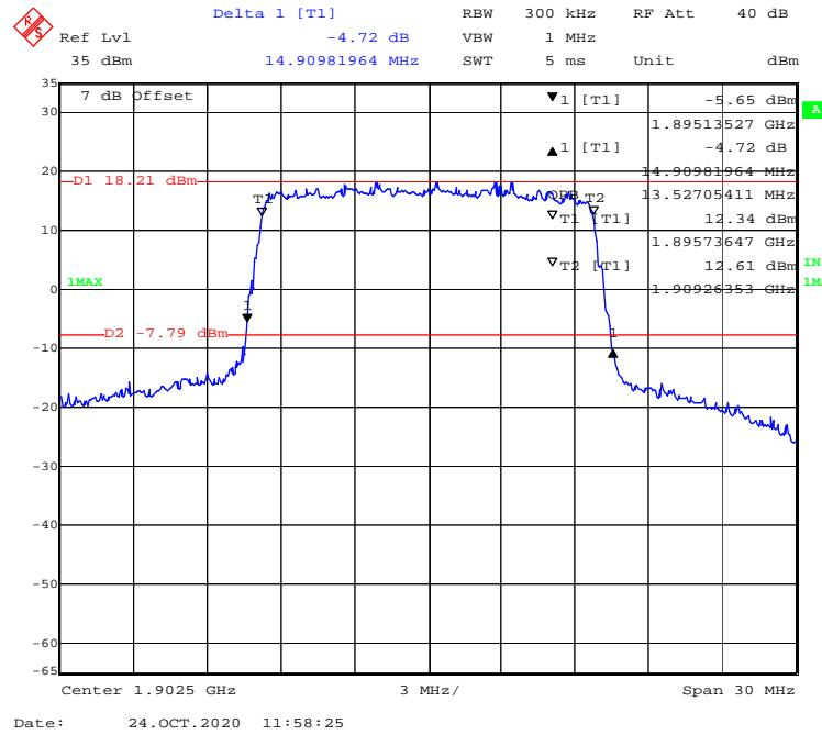
**16-QAM (20 MHz) - 99% Occupied & 26 dB Emissions Bandwidth, High channel**
