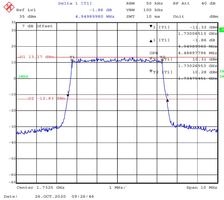
**16-QAM (10 MHz) - 99% Occupied & 26 dB Emissions Bandwidth, Middle channel**
