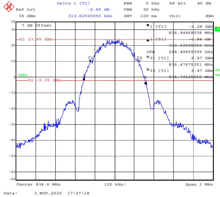
**99% Occupied & 26 dB Emissions Bandwidth for EGPRS (GMSK) High channel**
