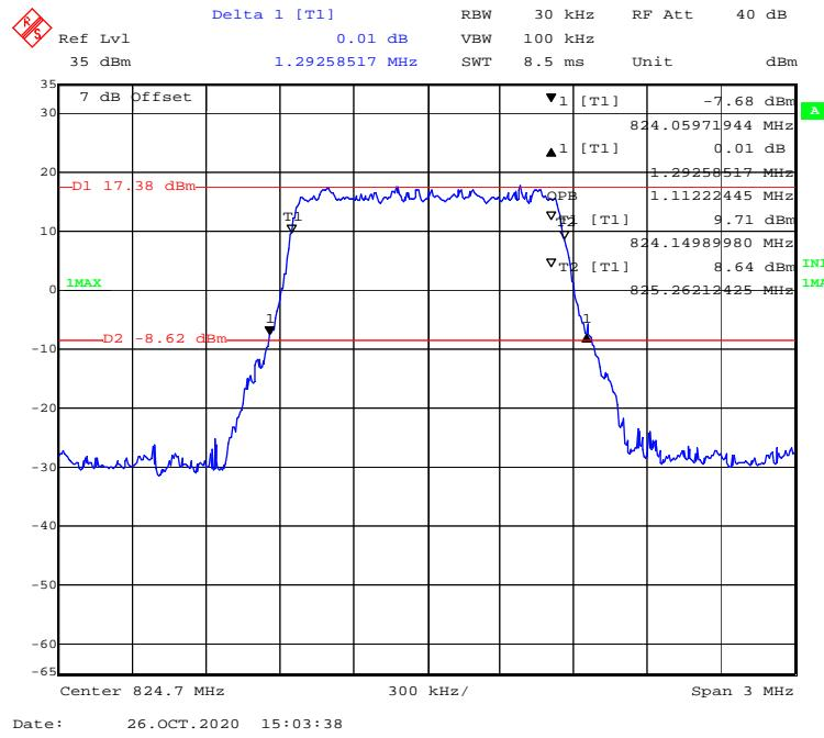
**QPSK (3.0 MHz) - 99% Occupied & 26 dB Emissions Bandwidth, Low channel**
