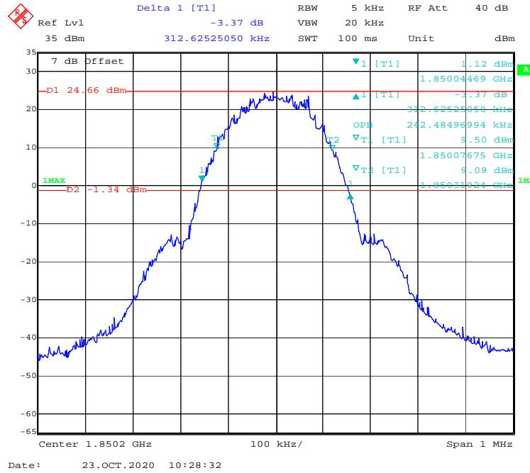
**99% Occupied & 26 dB Emissions Bandwidth for GSM (GMSK) Middle channel**
