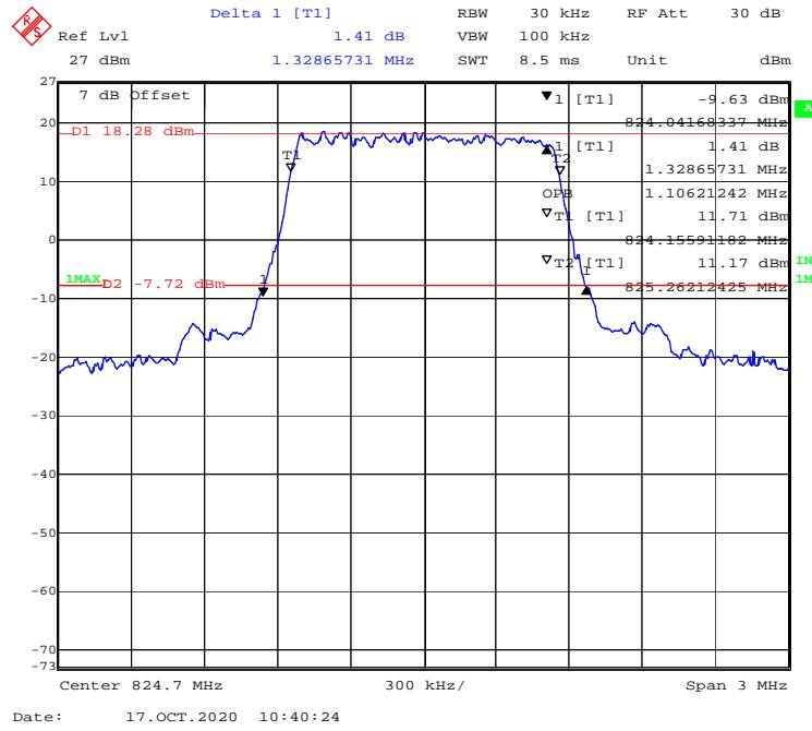
**1xRTT mode, 99% Occupied & 26 dB Emissions Bandwidth Middle channel**
