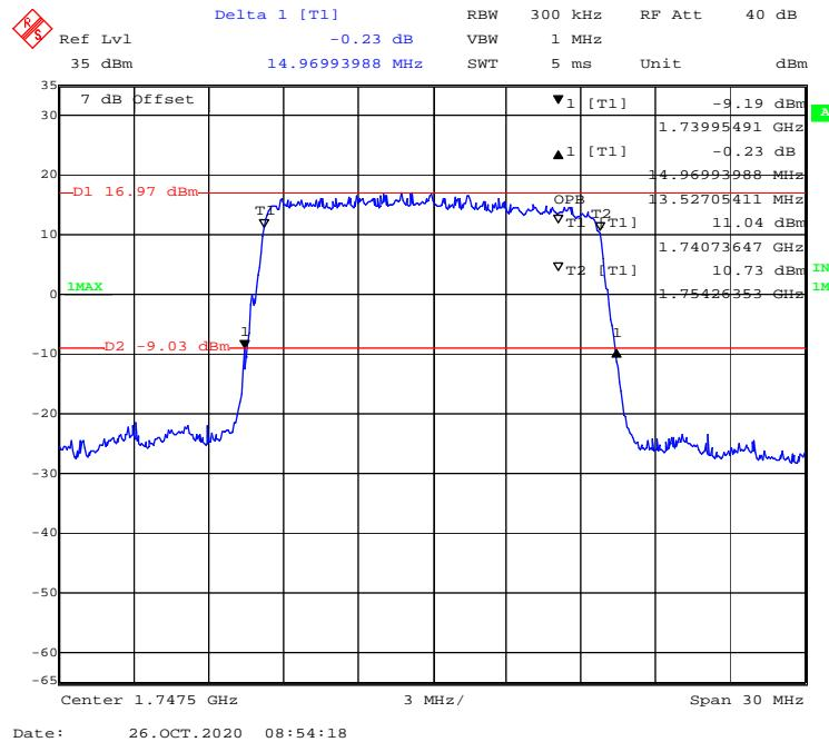
**QPSK (20 MHz) - 99% Occupied & 26 dB Emissions Bandwidth, High channel**
