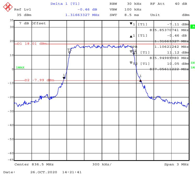
**16-QAM (3.0 MHz) - 99% Occupied & 26 dB Emissions Bandwidth, Middle channel**
