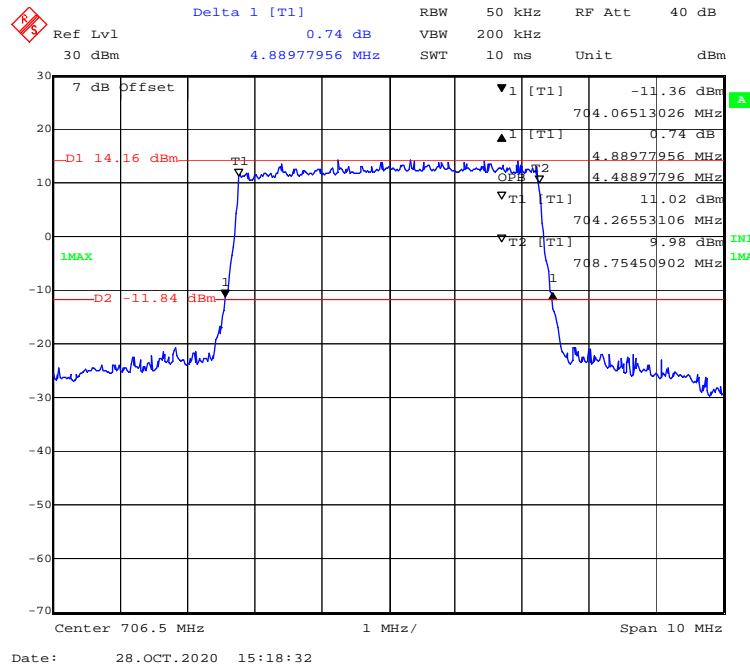
**16-QAM (10 MHz) - 99% Occupied & 26 dB Emissions Bandwidth, Low channel**
