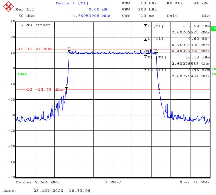
**16-QAM (10 MHz) - 99% Occupied & 26 dB Emissions Bandwidth, Middle channel**
