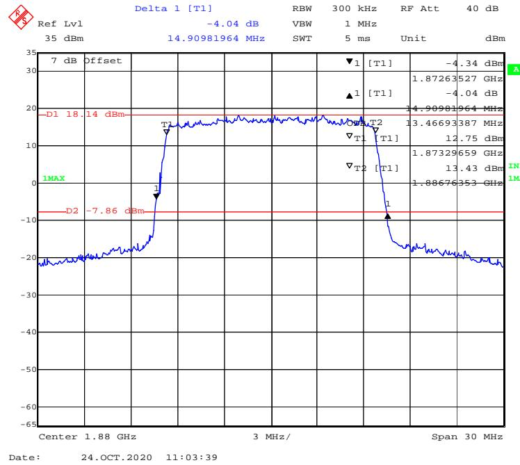
**QPSK (20 MHz) - 99% Occupied & 26 dB Emissions Bandwidth, Middle channel**
