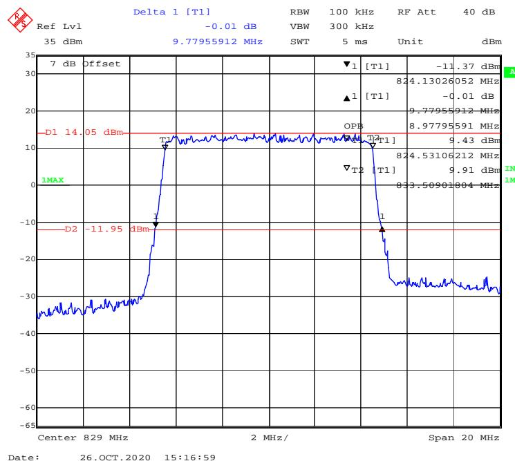
**QPSK (1.4 MHz) - 99% Occupied & 26 dB Emissions Bandwidth, Middle channel**
