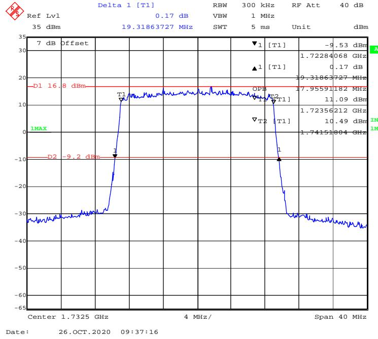
**QPSK (1.4 MHz) - 99% Occupied & 26 dB Emissions Bandwidth, High channel**
