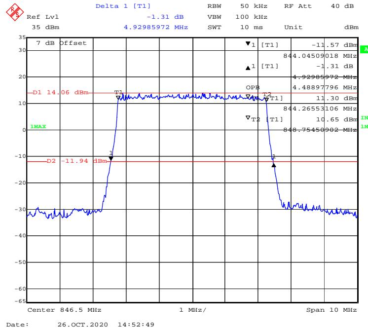
**16-QAM (10.0 MHz) - 99% Occupied & 26 dB Emissions Bandwidth, High channel**
