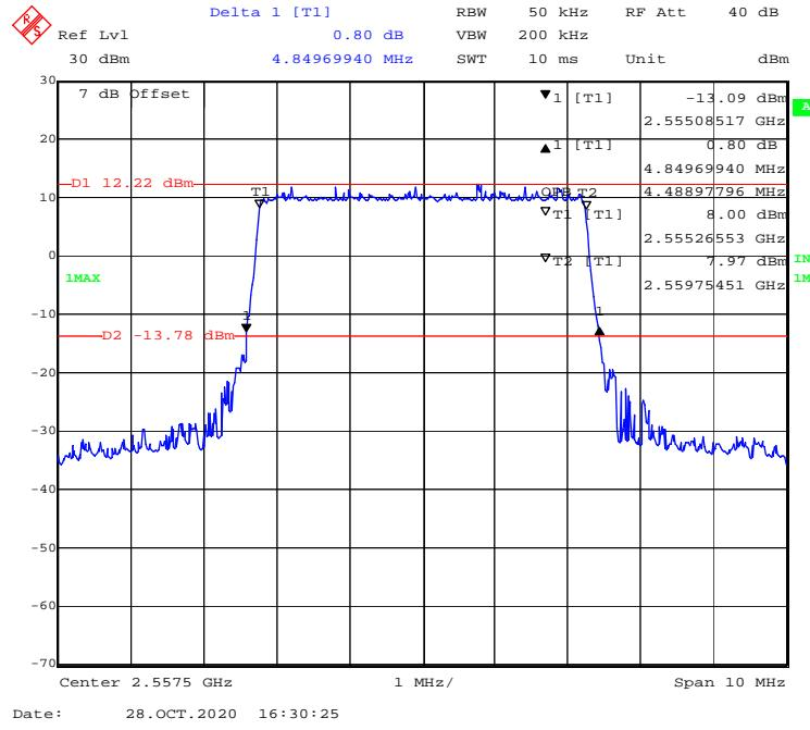
**QPSK (10 MHz) - 99% Occupied & 26 dB Emissions Bandwidth, Low channel**
