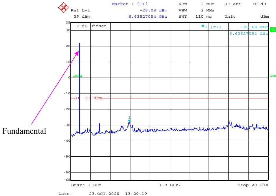
**30 MHz – 1GHz WCDMA (HSDPA) Mode , Middle channel**
