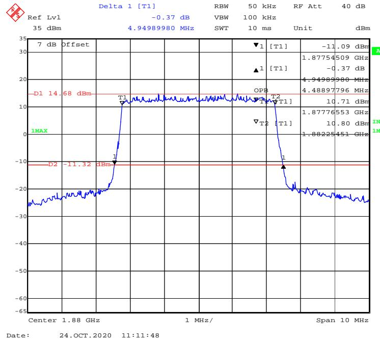
**16-QAM (10 MHz) - 99% Occupied & 26 dB Emissions Bandwidth, Middle channel**
