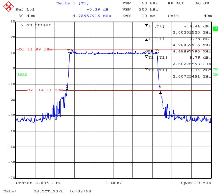
**QPSK (10 MHz) - 99% Occupied & 26 dB Emissions Bandwidth, Middle channel**
