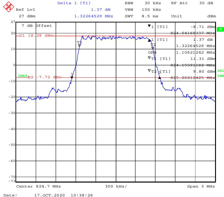
**EVDO mode, 99% Occupied & 26 dB Emissions Bandwidth Middle channel**
