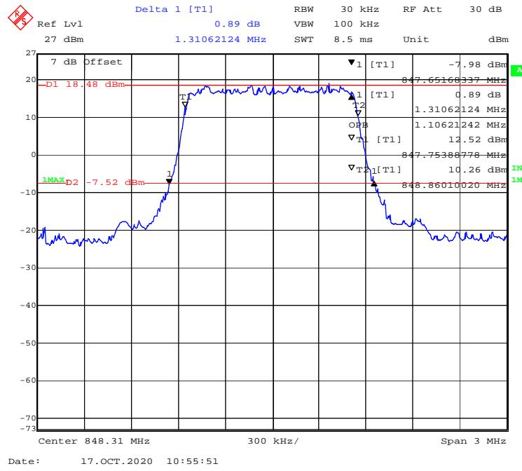
**1xRTT mode, 99% Occupied & 26 dB Emissions Bandwidth Low channel**
