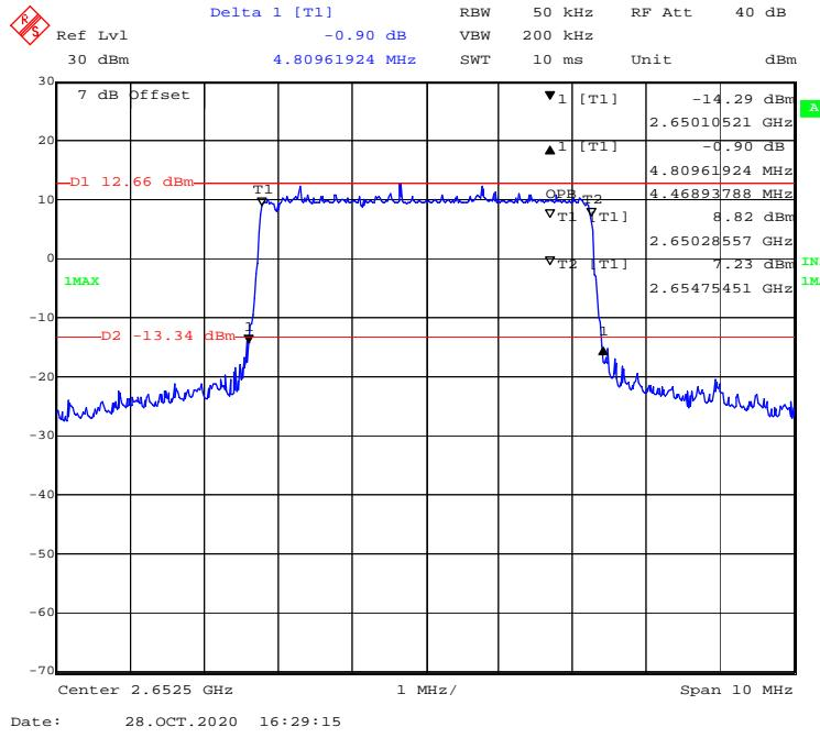
**QPSK (10 MHz) - 99% Occupied & 26 dB Emissions Bandwidth, High channel**
