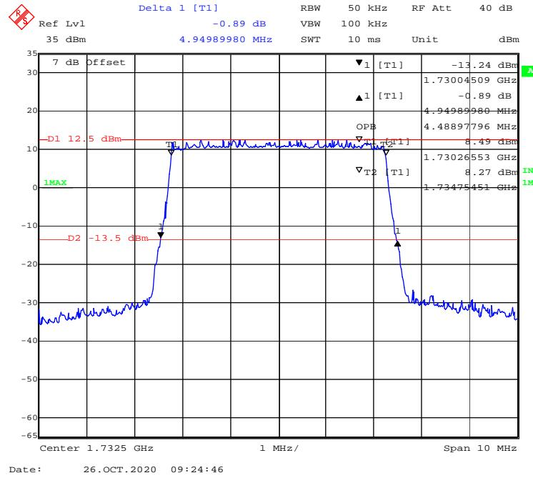
**QPSK (10 MHz) - 99% Occupied & 26 dB Emissions Bandwidth, Middle channel**
