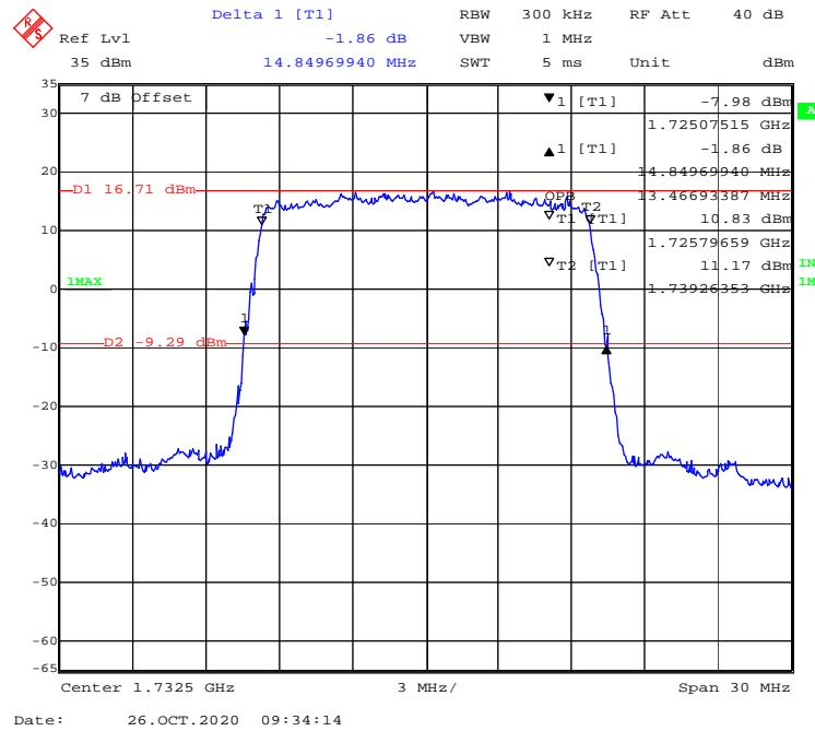
**16-QAM (20 MHz) - 99% Occupied & 26 dB Emissions Bandwidth, Middle channel**
