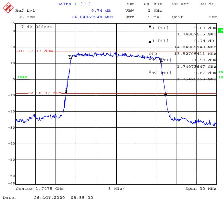
**16-QAM (20 MHz) - 99% Occupied & 26 dB Emissions Bandwidth, High channel**
