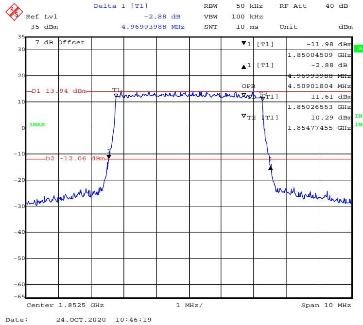
**16-QAM (10 MHz) - 99% Occupied & 26 dB Emissions Bandwidth, Low channel**
