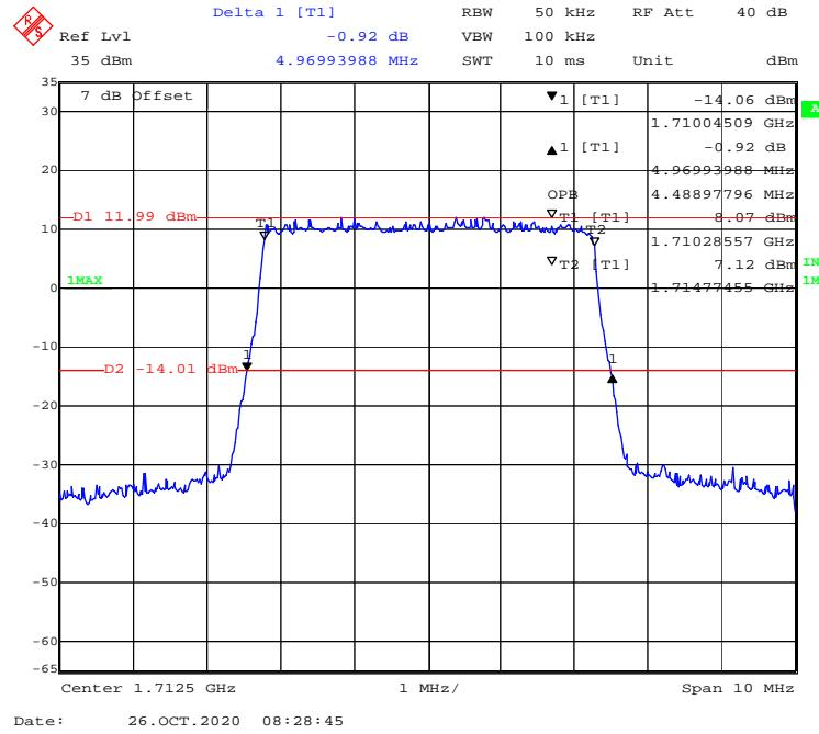
**QPSK (10 MHz) - 99% Occupied & 26 dB Emissions Bandwidth, Low channel**
