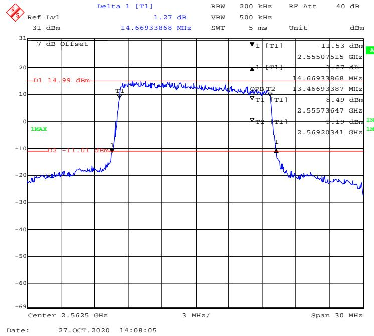
**16-QAM (20 MHz) - 99% Occupied & 26 dB Emissions Bandwidth, High channel**
