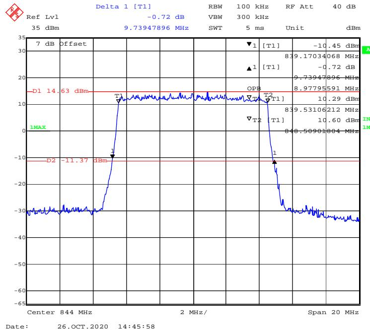
**16-QAM (1.4 MHz) - 99% Occupied & 26 dB Emissions Bandwidth, Low channel**
