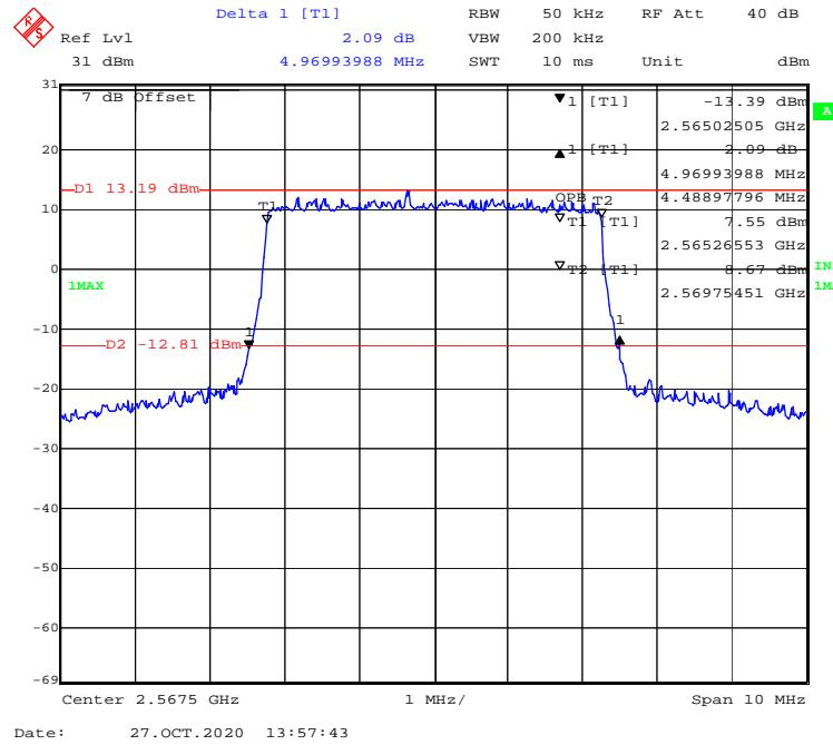
**16-QAM (10 MHz) - 99% Occupied & 26 dB Emissions Bandwidth, High channel**
