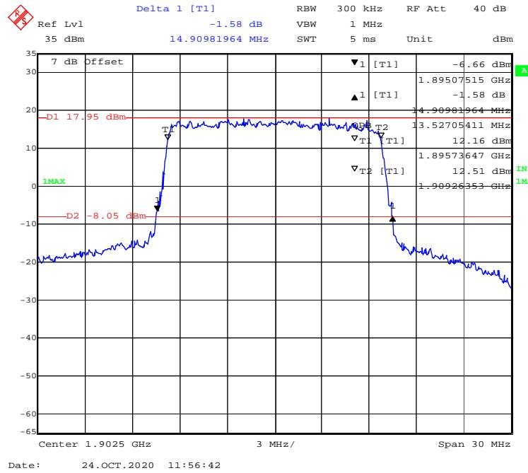
**QPSK (20 MHz) - 99% Occupied & 26 dB Emissions Bandwidth, High channel**
