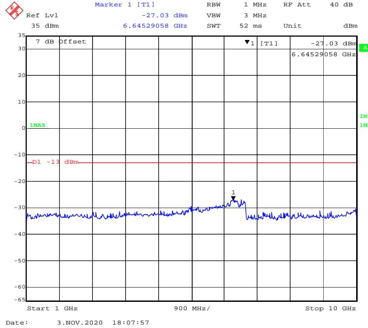
**WCDMA Band V:****30 MHz – 1GHz WCDMA (Rel 99) Mode, Low channel**
