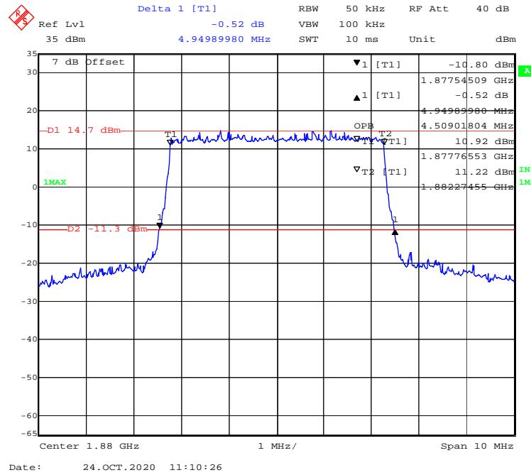
**QPSK (10MHz) - 99% Occupied & 26 dB Emissions Bandwidth, Middle channel**
