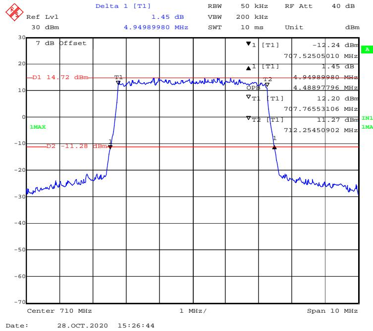
**QPSK (10MHz) - 99% Occupied & 26 dB Emissions Bandwidth, Middle channel**
