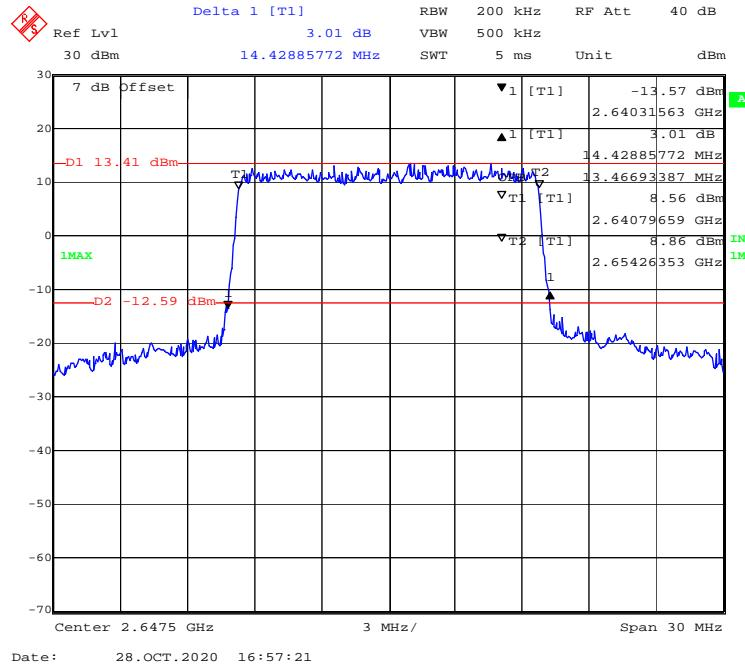
**QPSK (20 MHz) - 99% Occupied & 26 dB Emissions Bandwidth, High channel**
