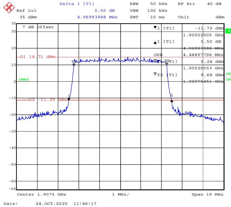
**QPSK (10MHz) - 99% Occupied & 26 dB Emissions Bandwidth, High channel**
