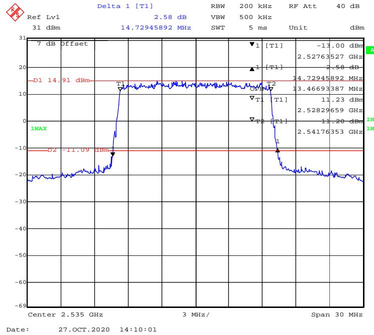
**16-QAM (20 MHz) - 99% Occupied & 26 dB Emissions Bandwidth, Middle channel**
