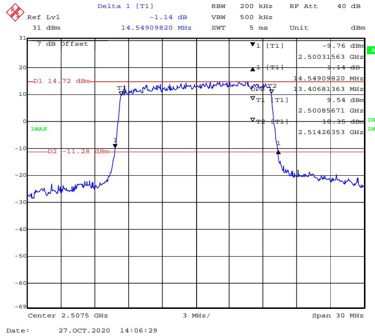
**16-QAM (20 MHz) - 99% Occupied & 26 dB Emissions Bandwidth, Low channel**
