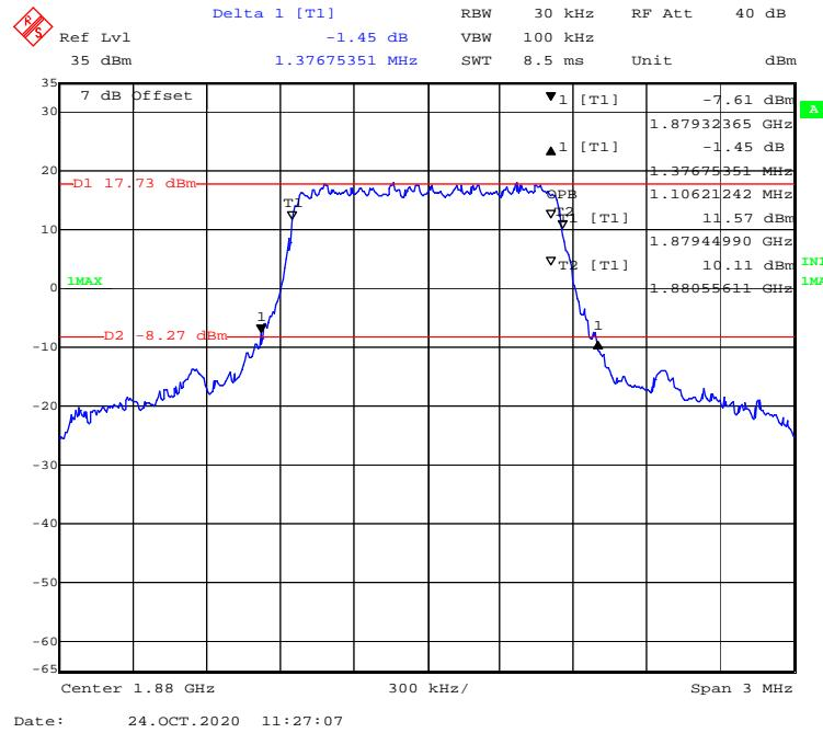
**QPSK (3 MHz) - 99% Occupied & 26 dB Emissions Bandwidth, Middle channel**
