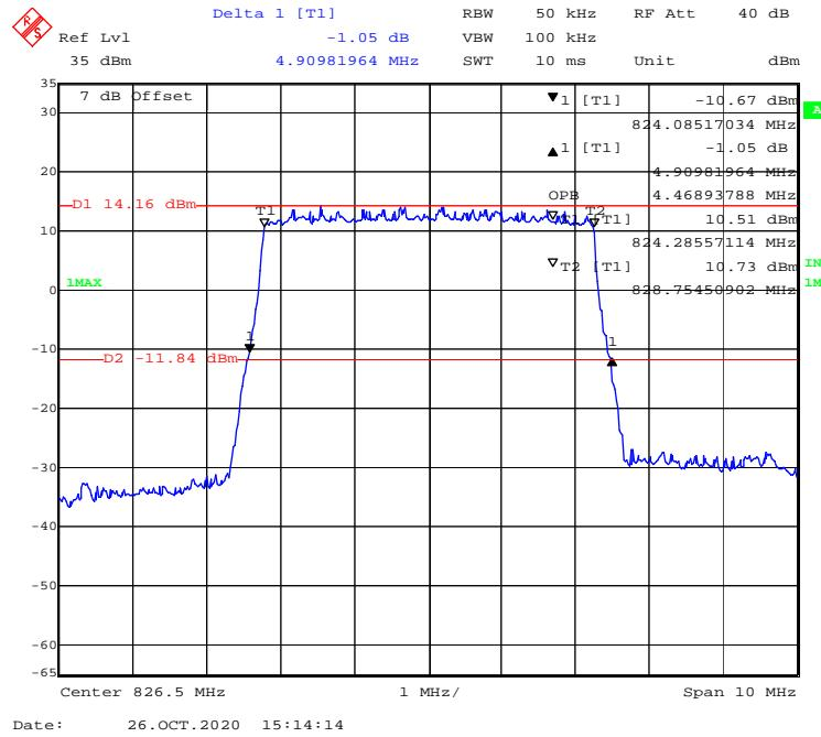
**16-QAM (10.0 MHz) - 99% Occupied & 26 dB Emissions Bandwidth, Low channel**
