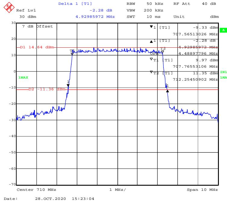
**16-QAM (10 MHz) - 99% Occupied & 26 dB Emissions Bandwidth, Middle channel**
