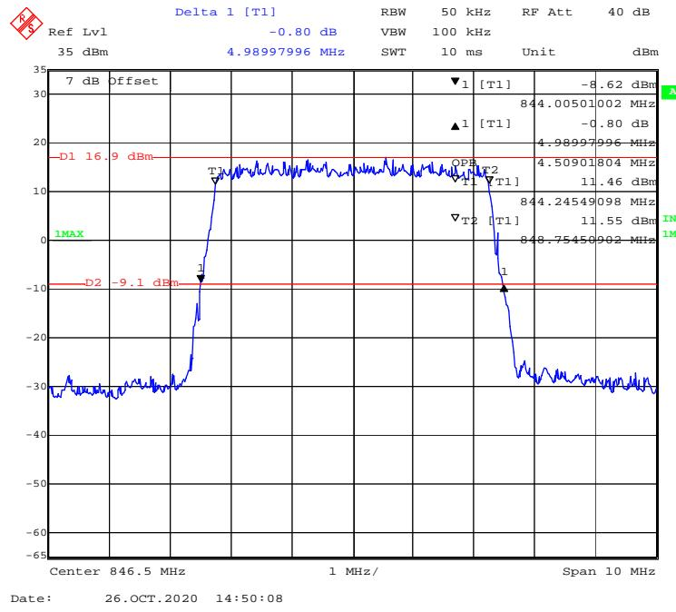
**QPSK (10.0 MHz) - 99% Occupied & 26 dB Emissions Bandwidth, High channel**
