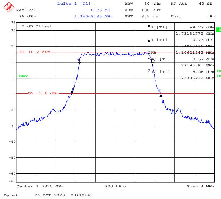
**16-QAM (3 MHz) - 99% Occupied & 26 dB Emissions Bandwidth, Middle channel**
