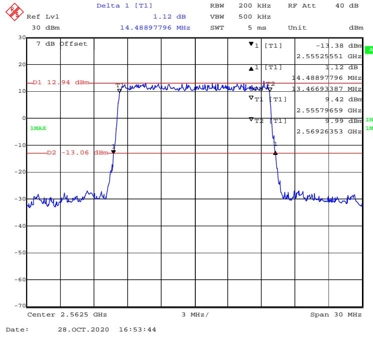
**16-QAM (20 MHz) - 99% Occupied & 26 dB Emissions Bandwidth, Low channel**
