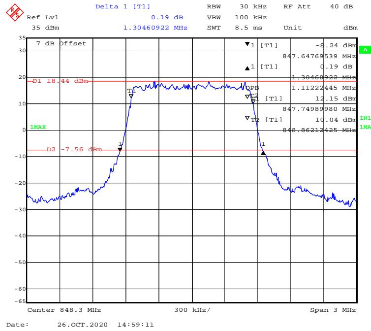
**QPSK (3.0 MHz) - 99% Occupied & 26 dB Emissions Bandwidth, High channel**
