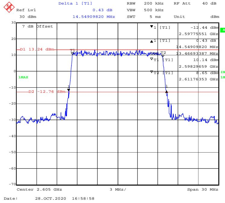
**QPSK (20 MHz) - 99% Occupied & 26 dB Emissions Bandwidth, Middle channel**
