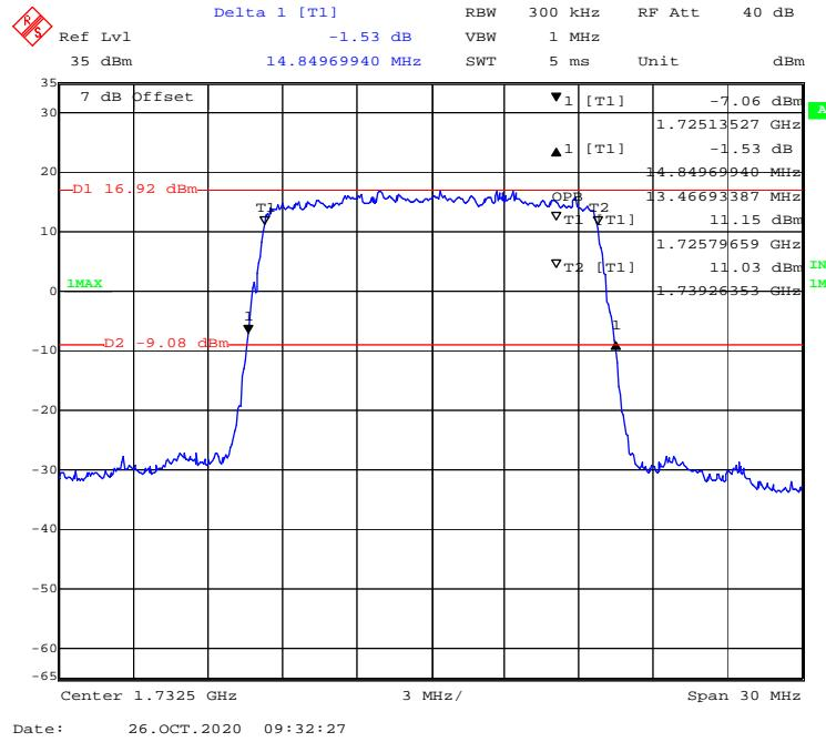
**QPSK (20 MHz) - 99% Occupied & 26 dB Emissions Bandwidth, Middle channel**
