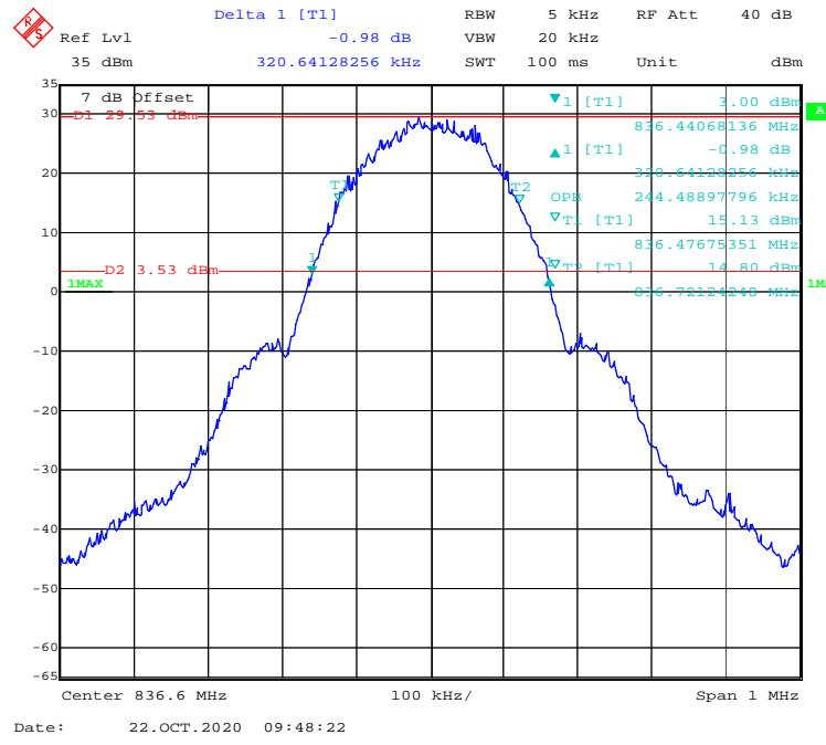
**99% Occupied & 26 dB Emissions Bandwidth for GPRS (GMSK) High channel**
