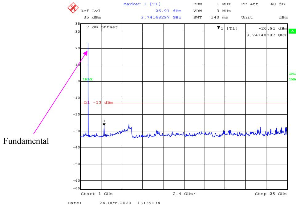
**30 MHz - 1 GHz (5 MHz, 16-QAM, Middle Channel)**
