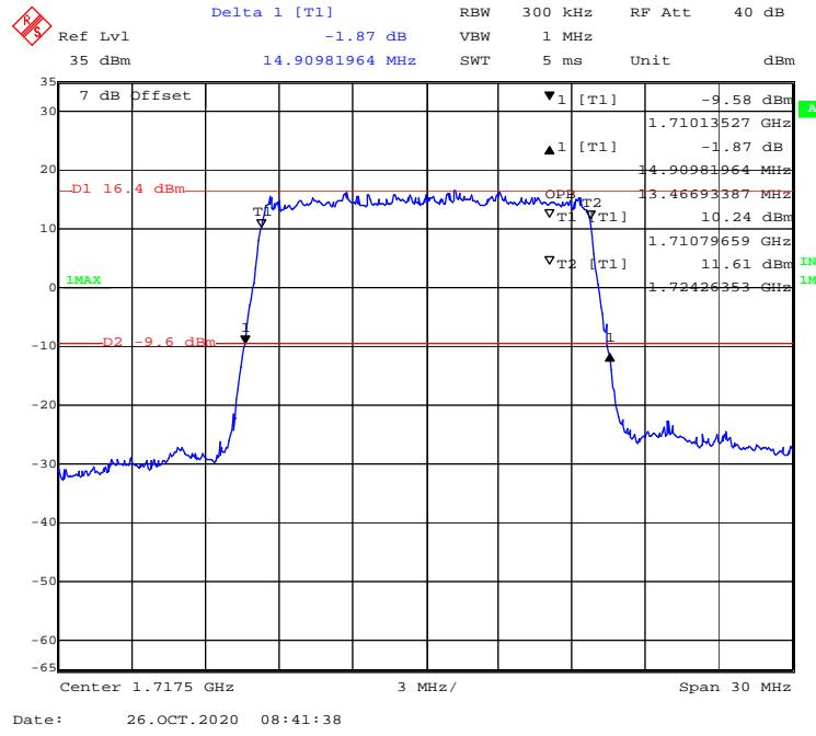
**QPSK (20 MHz) - 99% Occupied & 26 dB Emissions Bandwidth, Low channel**
