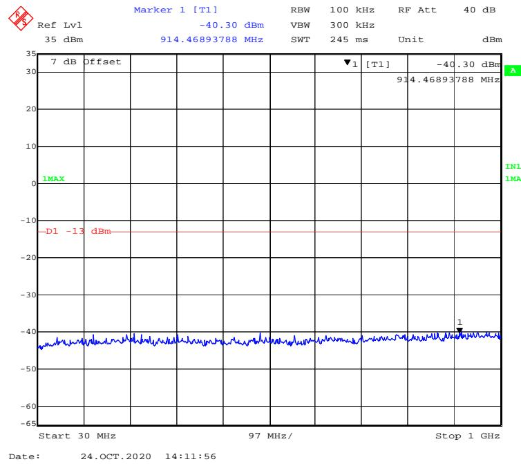
**1 GHz – 25 GHz (20 MHz, 16-QAM, Middle Channel)**
