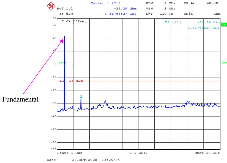
**30 MHz – 1GHz WCDMA (HSUPA) Mode , High channel**
