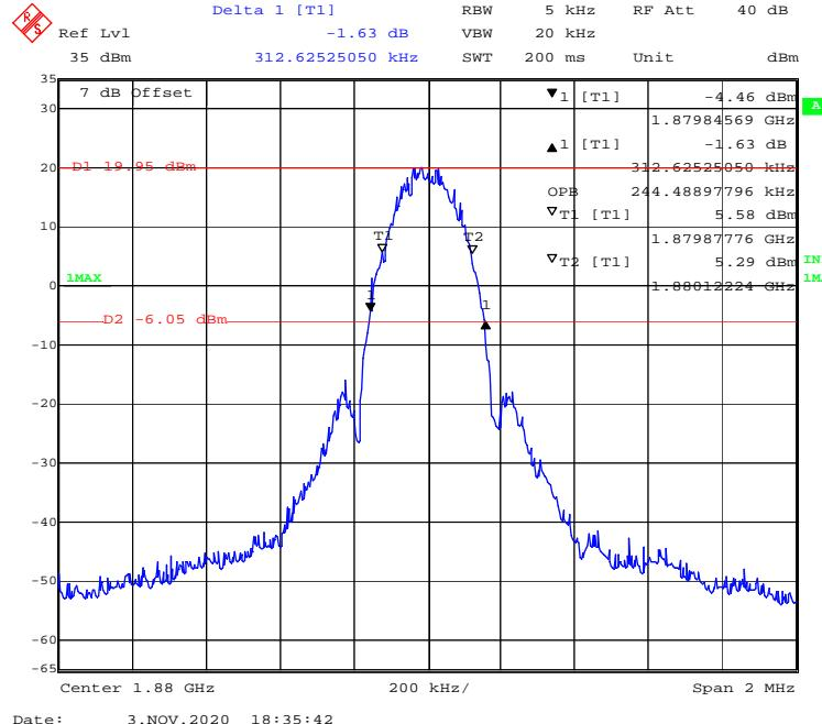
**99% Occupied & 26 dB Emissions Bandwidth for EGPRS (8PSK) High channel**
