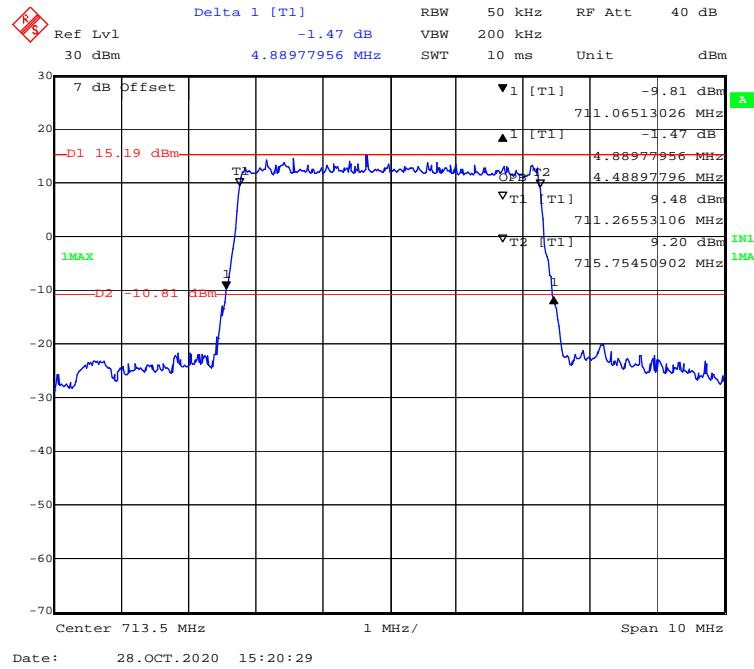
**16-QAM (10 MHz) - 99% Occupied & 26 dB Emissions Bandwidth, High channel**
