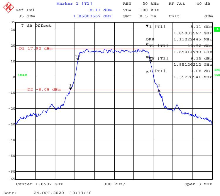
**16-QAM (3 MHz) - 99% Occupied & 26 dB Emissions Bandwidth, Low channel**
