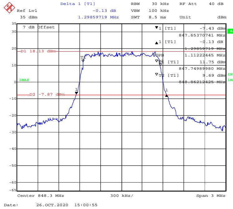
**16-QAM (3.0 MHz) - 99% Occupied & 26 dB Emissions Bandwidth, High channel**
