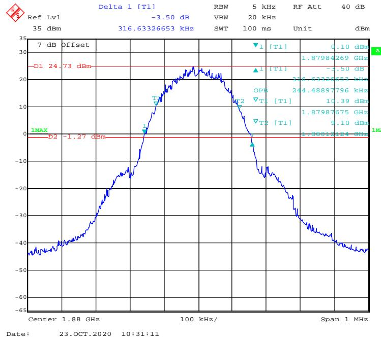
**99% Occupied & 26 dB Emissions Bandwidth for GPRS (GMSK) High channel**
