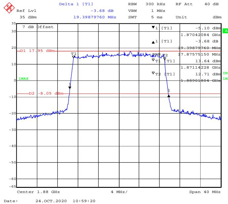
**QPSK (1.4 MHz) - 99% Occupied & 26 dB Emissions Bandwidth, High channel**
