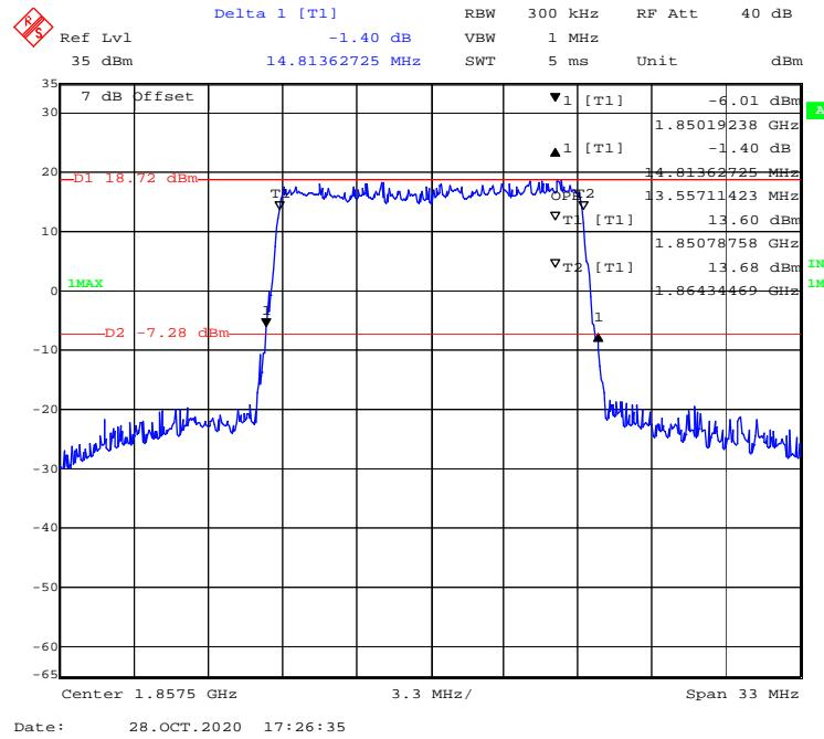
**QPSK (20 MHz) - 99% Occupied & 26 dB Emissions Bandwidth, Low channel**
