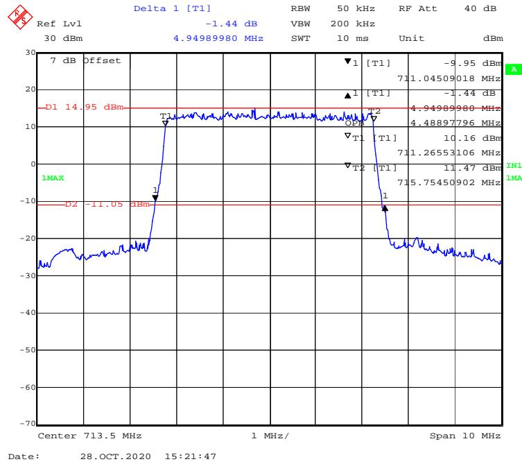
**QPSK (10MHz) - 99% Occupied & 26 dB Emissions Bandwidth, High channel**
