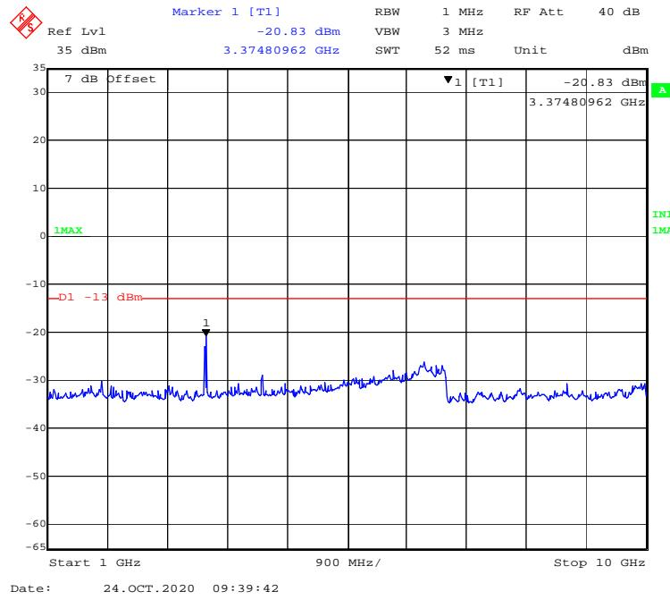
**30 MHz – 1GHz WCDMA (Rel 99) Mode, Middle channel**
