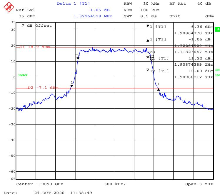
**16-QAM (3 MHz) - 99% Occupied & 26 dB Emissions Bandwidth, High channel**
