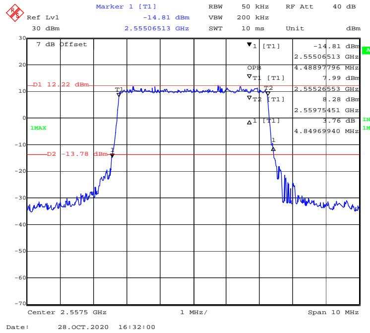
**16-QAM (10 MHz) - 99% Occupied & 26 dB Emissions Bandwidth, Low channel**
