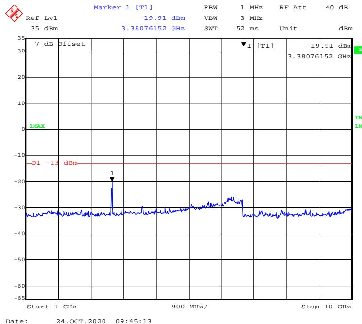
**30 MHz – 1GHz WCDMA (HSDPA) Mode, High channel**
