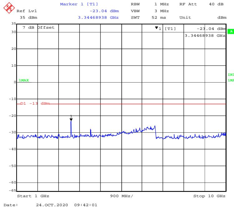
**30 MHz – 1GHz WCDMA (Rel 99) Mode, High channel**
