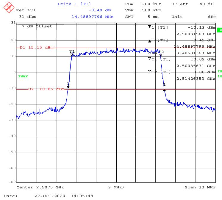
**QPSK (20 MHz) - 99% Occupied & 26 dB Emissions Bandwidth, Low channel**
