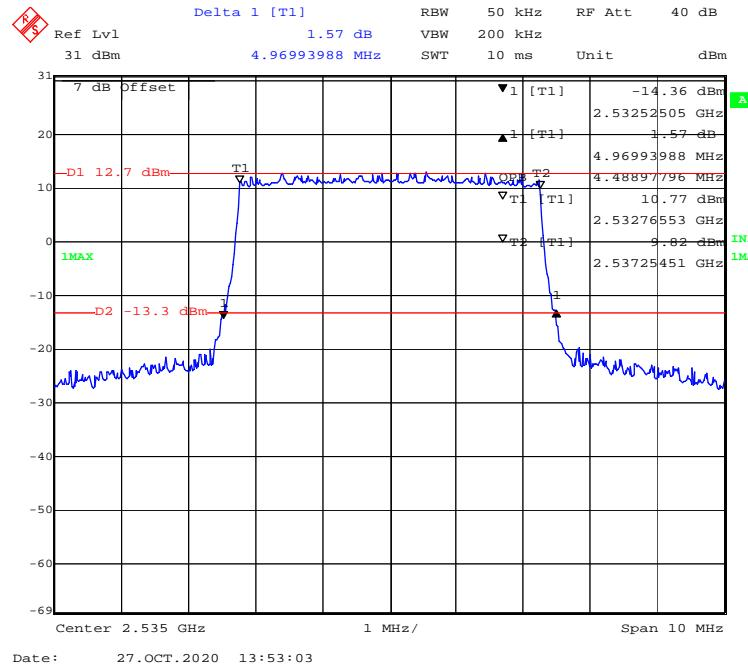
**16-QAM (10 MHz) - 99% Occupied & 26 dB Emissions Bandwidth, Middle channel**
