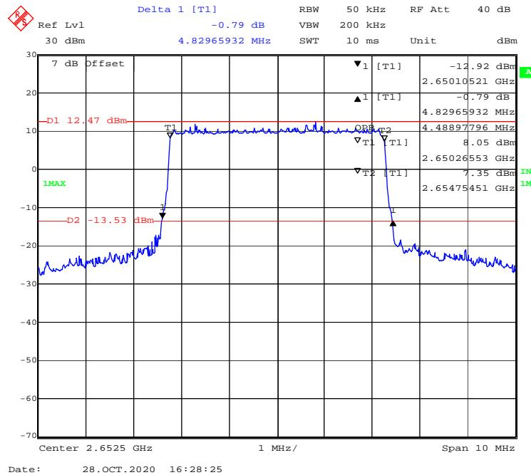
**16-QAM (10 MHz) - 99% Occupied & 26 dB Emissions Bandwidth, High channel**
