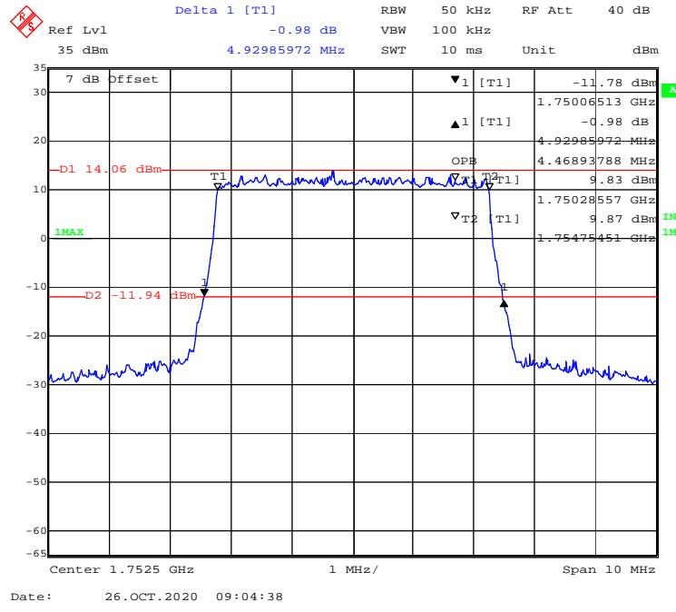
**16-QAM (10 MHz) - 99% Occupied & 26 dB Emissions Bandwidth, High channel**
