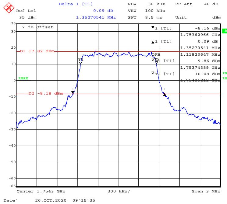
**16-QAM (3 MHz) - 99% Occupied & 26 dB Emissions Bandwidth, High channel**
