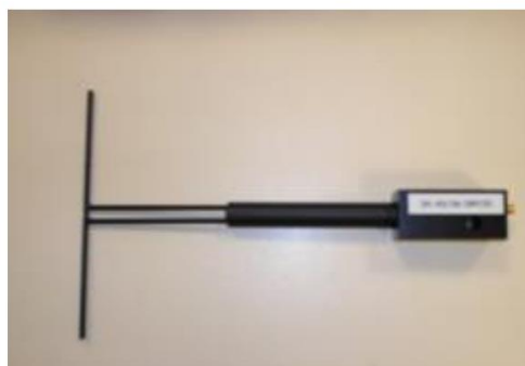
Figure 1 – Satimo COMOSAR Validation Dipole
