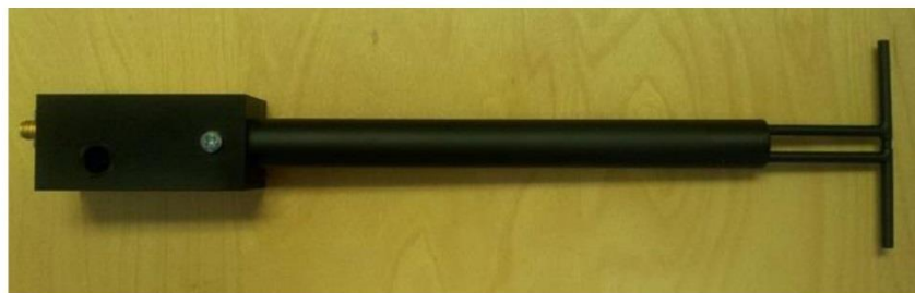
Figure 1 – MVG COMOSAR Validation Dipole
