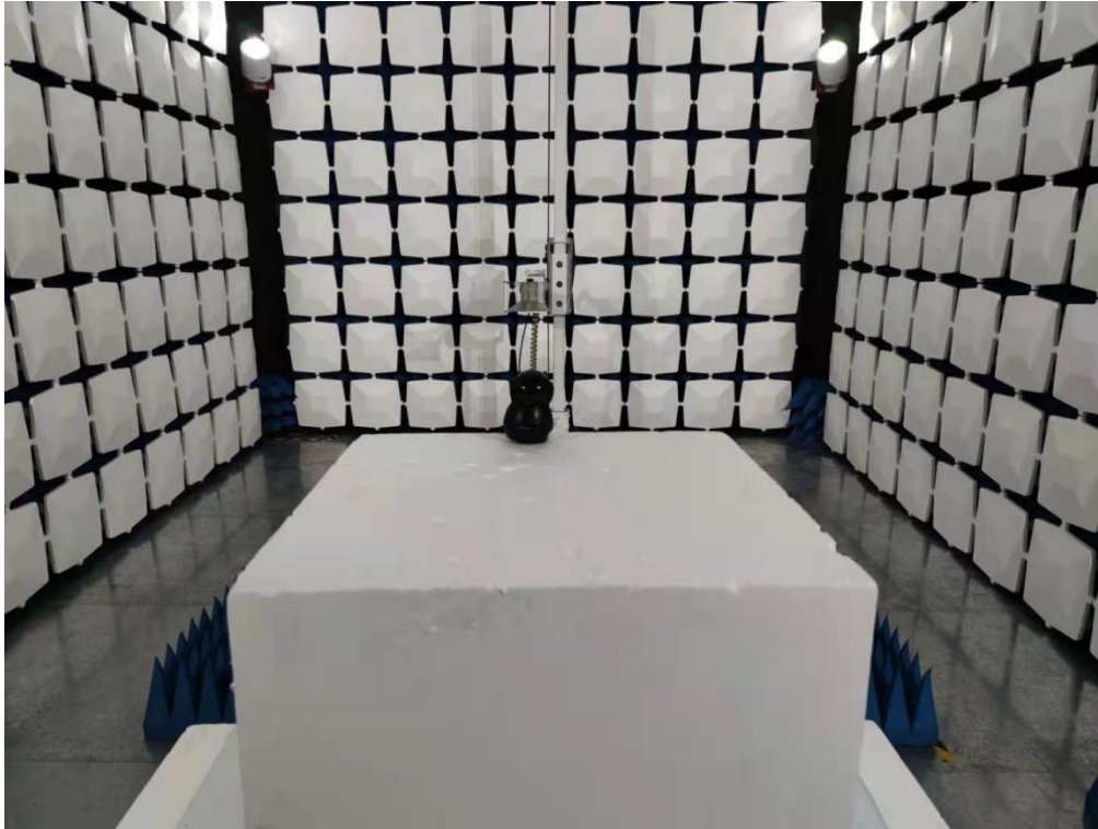
Above 1GHz for radiated emission test setup
